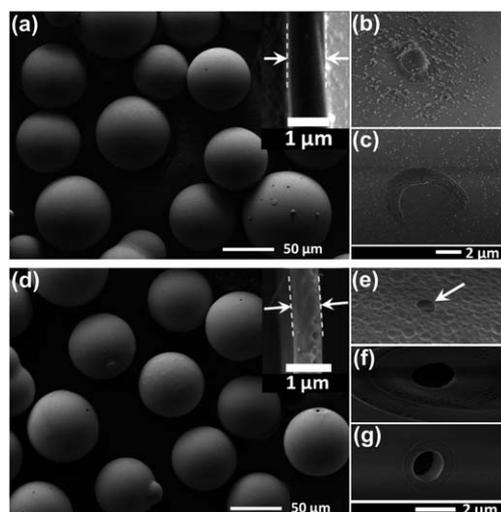
**Fig. 3** (a) The overview of the original GBs in 63–90  $\mu\text{m}$  after water deposition; (b) and (c) the defects in the shell; (d) the etched GBs in 63–90  $\mu\text{m}$  after water deposition; (e)–(g) the through-holes etched in the shell. The insets in (a) and (d) show the cross-sectional thickness of the original and etched GB, respectively.
