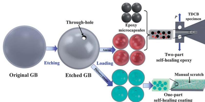
**Fig. 1** The schematic illustration (not to scale) of the whole experimental process, including the etching of GBs, the loading of the etched GBs, and the sample preparation of two-part self-healing epoxy and one-part self-healing coating. The healing performances of self-healing epoxy and coating were characterized using the TDCB specimen (top right image) and the coated metal substrate (bottom right image), respectively.
