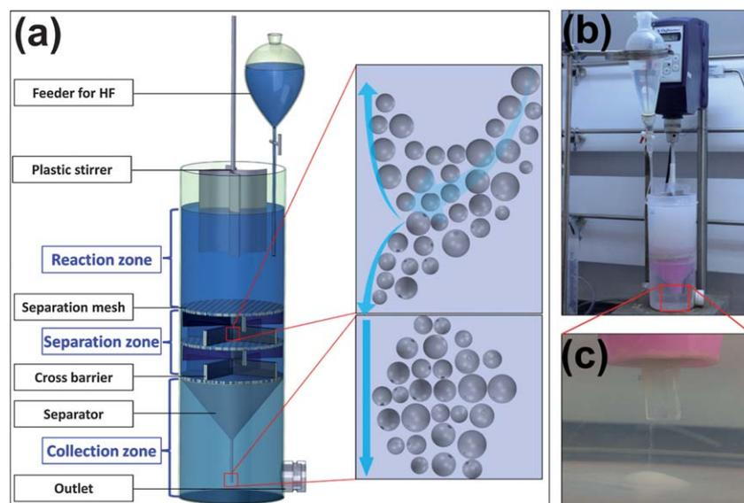
**Fig. 2** (a) The schematic configuration of the specially designed etching system with interconnected segmented zones; (b) the real image of the reaction system during etching; (c) the enlarged tip in the collection zone showing the deposition of the well-etched GBs.
