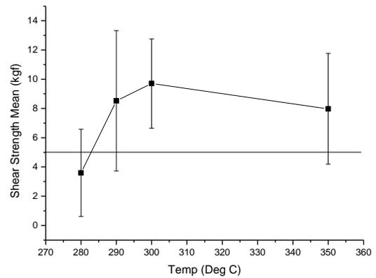
Fig. 2 Shear strength test results with varying bonding temperature
