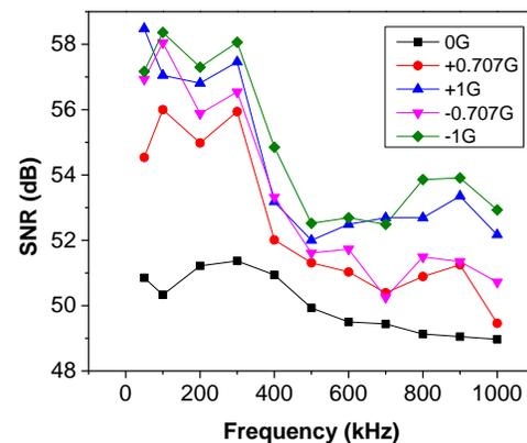
**Fig. 21** SNR as a function of carrier frequency at various  $g$  orientations, when carrier amplitude is 1Vpp.
