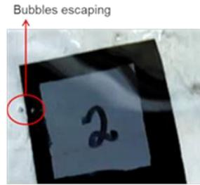
**Fig. 6** Example of a stream of bubbles observed in gross leak test
