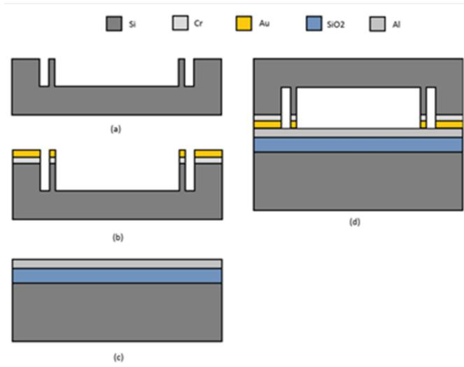
**Fig. 5** Schematics of the formation of sealed cavity for helium leak rate detection: (a) forming of cavities, seal rings and air channel using DRIE etching; (b) sequential deposition of Cr layer and Au bonding layer; (c) deposition of SiO<sub>2</sub> isolation and Al bonding layer; (d) Au-Al thermo-compression bonding of the cavity wafer to the capping wafer.
