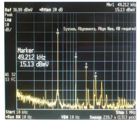
**Fig. 20** FFT spectrum showing fundamental peak at the carrier frequency and higher order harmonics at integer multiples of carrier frequency.
