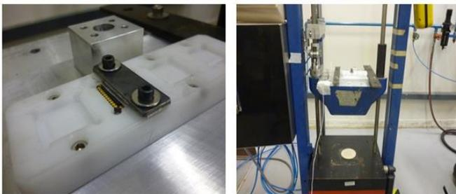
**Fig. 23** Setup for the 500g shock test. The chip is subjected to a maximum vertical acceleration of 503.55g for a short duration of 1.03 ms for a total number of 10 times.
