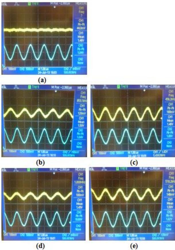
**Fig. 18** The gain stage output (yellow, upper trace) when the excitation carrier amplitude is 1Vpp (blue, lower trace) at 50kHz frequency and the bonded chip is tilted at: (a) 0g, (b) -0.707g, (c) -1g, (d) +0.707g and (e) +1g orientation. Acceleration at a tilt angle  $\theta$  is given by  $g \sin(\theta)$ .
