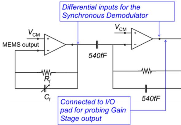
**Fig. 12** Schematic diagram of the low noise, band-pass gain stage which consists of two single-ended output amplifiers based on folded-cascode architecture. Pseudo-resistors are used in the feedback path of the amplifiers. Tunable feedback capacitance allows variable gain.
