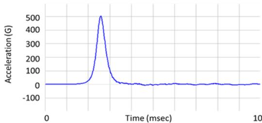
**Fig. 24** General control profile during the 500g and 1 ms mechanical shock test.
