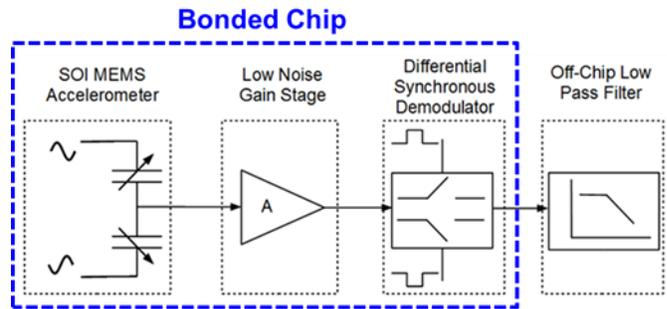
**Fig. 17** System block diagram for the bonded MEMS/CMOS microsystem. The MEMS and CMOS have been seamlessly integrated to form a single bonded chip. There is no wire-bonding from chip to chip. Chip to chip electrical connections are done using direct metal bonding without solder.
