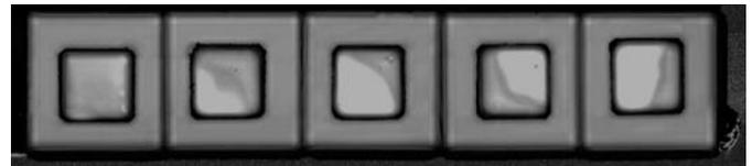
Fig. 3 Shear strength test results with varying bonding temperature C-SAM image of samples bonded at 290 $^{\circ}$ C
