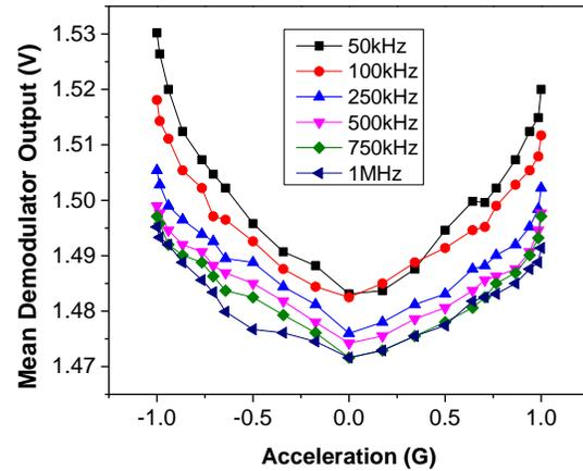
**Fig. 19** Variation in the mean demodulator output with  $g$  at various carrier frequencies for the bonded chip.
