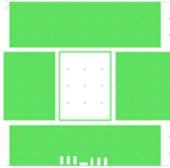
**Fig. 4** Seal cavity mask pattern for DRIE for hermetic test dies
