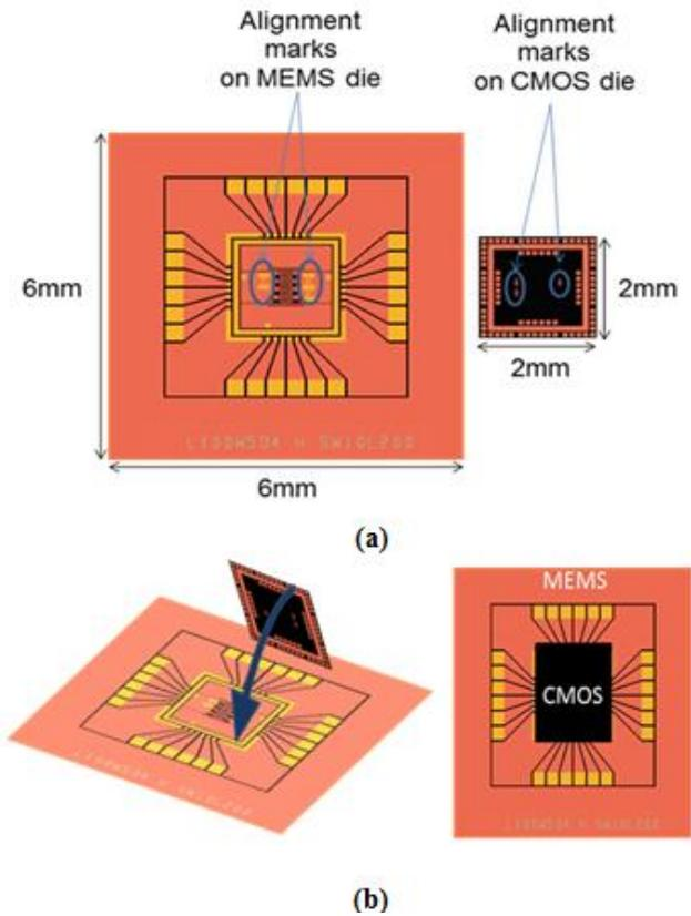
**Fig. 15** (a) The alignment marks on MEMS and CMOS die are used for orienting the dies before stacking. (b) The CMOS die is vertically stacked on top of MEMS die
