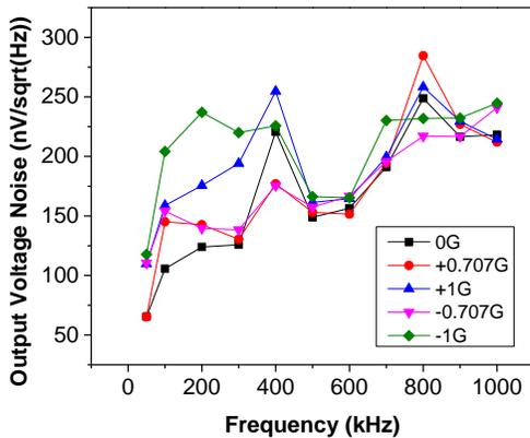
**Fig. 22** Output voltage noise as a function of carrier frequency at various g orientations, when carrier amplitude is 1Vpp.
