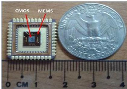
**Fig. 16** The CMOS chip is bonded face-to-face on the MEMS chip. The bonded chip is then wire bonded to the package for electrical testing. The vertically stacked CMOS and MEMS chip has a thickness of 1155µm.
