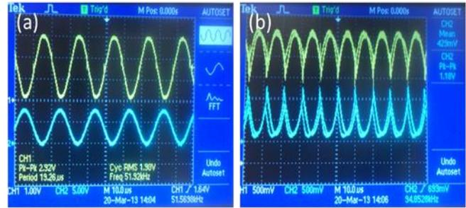
**Fig. 14** (a) The band-pass gain stage output (yellow, upper trace) during the standalone testing of the CMOS readout, when one of the carrier amplitude is 7.5Vpp (blue, lower trace) at 50 kHz frequency and 0g acceleration. (b) Fully-rectified sinusoids at the synchronous demodulator outputs, verifying that the readout is working as intended.
