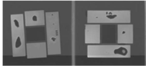
**Fig. 7** C-SAM image of hermetic test dies
