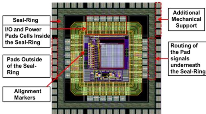
**Fig. 13** Die Micrograph of the readout circuit fabricated through MPW (0.35 $\mu$ m, 2P4M process). Key components are highlighted and specific ones are seal ring, mechanical support and alignment marks to assist the MEMS-CMOS bonding.
