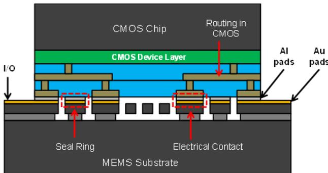
Fig. 1 3D stacking of MEMS and CMOS
