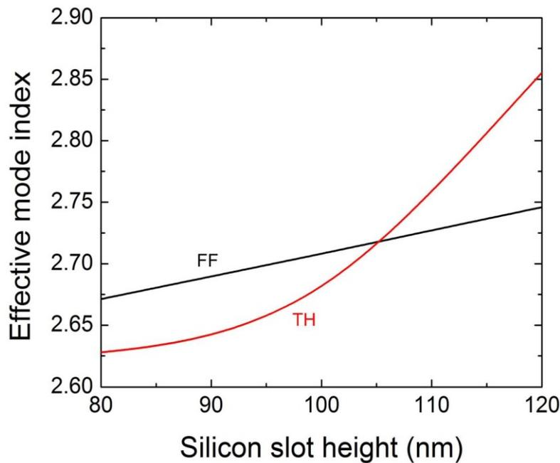
Figure 1. Effective mode indices of the zeroth mode at FF and the first mode at TH versus the silicon slot height with fixed  $w_1 = 40$  nm,  $h_1 = 400$  nm,  $w_2 = 140$  nm.
