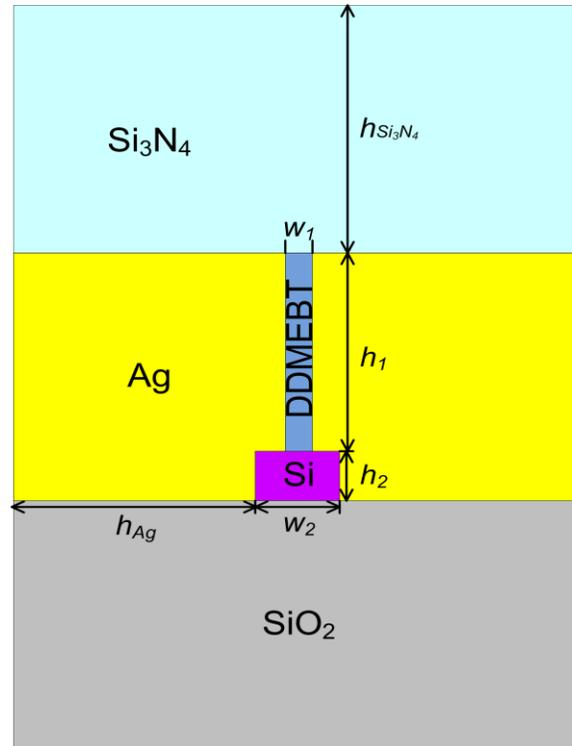
Figure 1. Cross-section view of the proposed double-asymmetric plasmonic slot waveguide (DAPSW).
