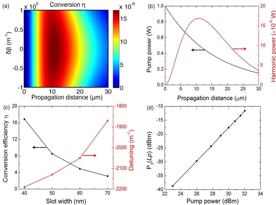
Figure 4. Fixed the pump power to be 1 W, (a) contour plot of the conversion efficiency with different  $\delta\beta$ , (b) optical powers of FF and TH over the propagation distance with  $\delta\beta = -3600$   $\text{m}^{-1}$ , (c) conversion efficiency and the corresponding detuning versus the slot width; (d) harmonic power versus the input pump power.
