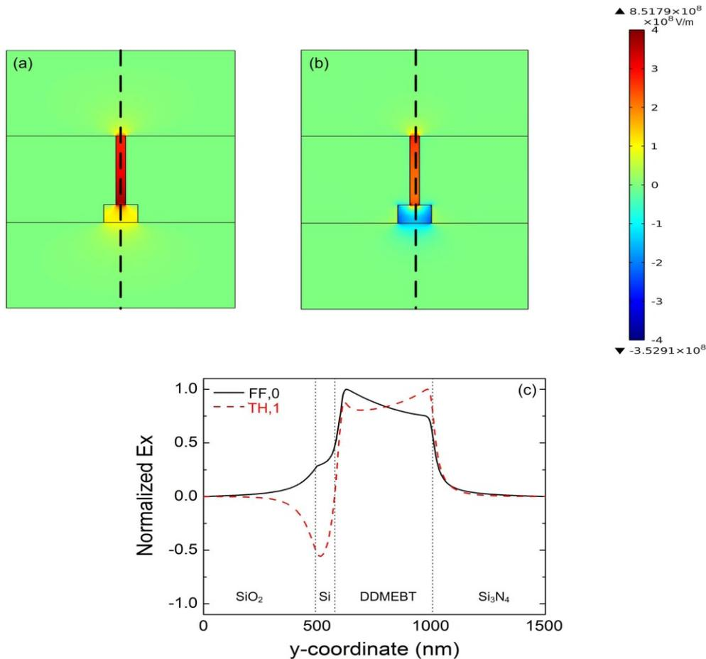
Figure 2. Major  $E_x$  profiles of (a) zeroth mode at FF and (b) first mode at TH; 1D  $E_x$  distributions of FF and TH at a cutline of (c)  $x = 0$  as the dash lines plotted in (a) (b). '0' stands for the zeroth mode, '1' stands for the first mode.
