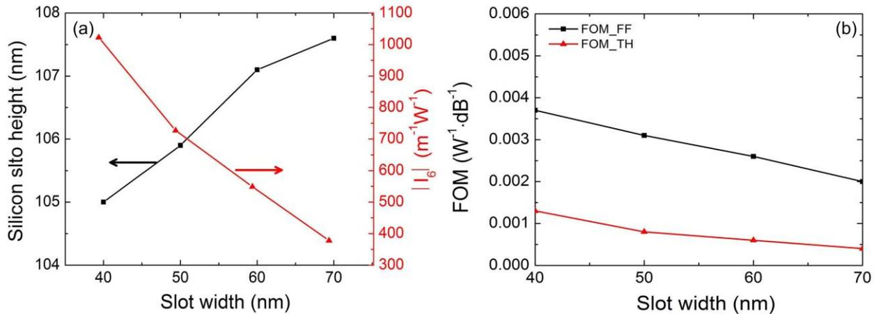
Figure 3. Silicon slot height along with the corresponding  $|I_6|$  values versus the slot width satisfying PMC, (b) FOMs as a function of the slot width at different PMCs.
