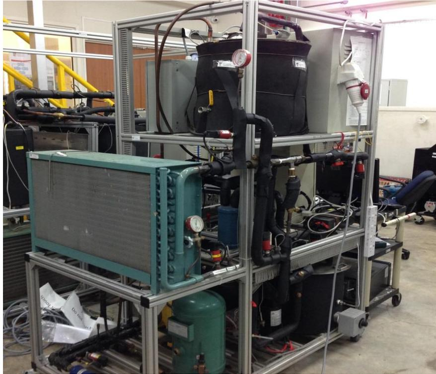
Fig. 4 Photograph of the ejector refrigeration system
