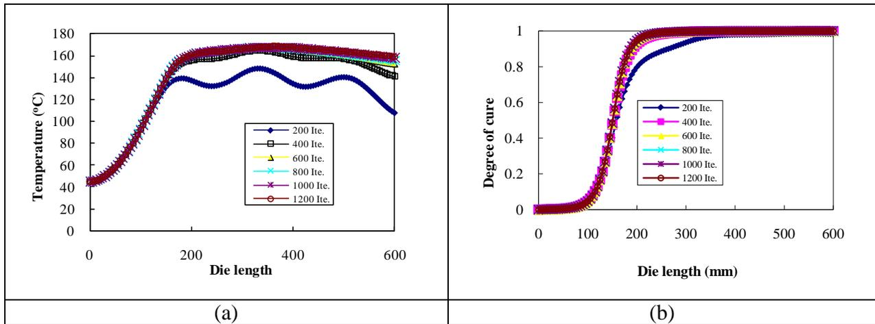
Figure 4, (a) temperature and (b) degree of cure profiles along centerline (node 10018 in Fig. 2) of GFRP facesheet of sandwich pultrudate.
