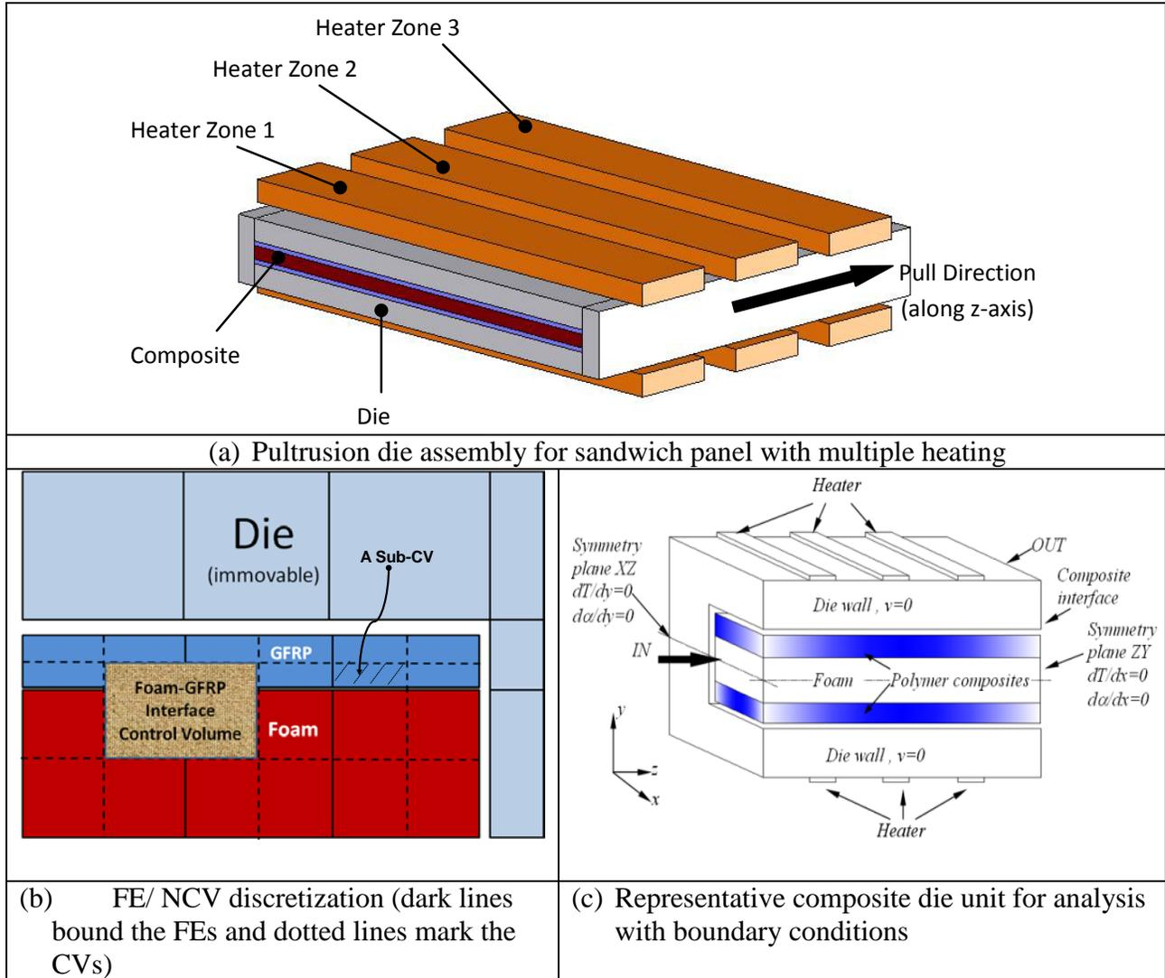
Figure 1 Geometric representation and FE/NCV discretization of pultrusion die-composites assembly
