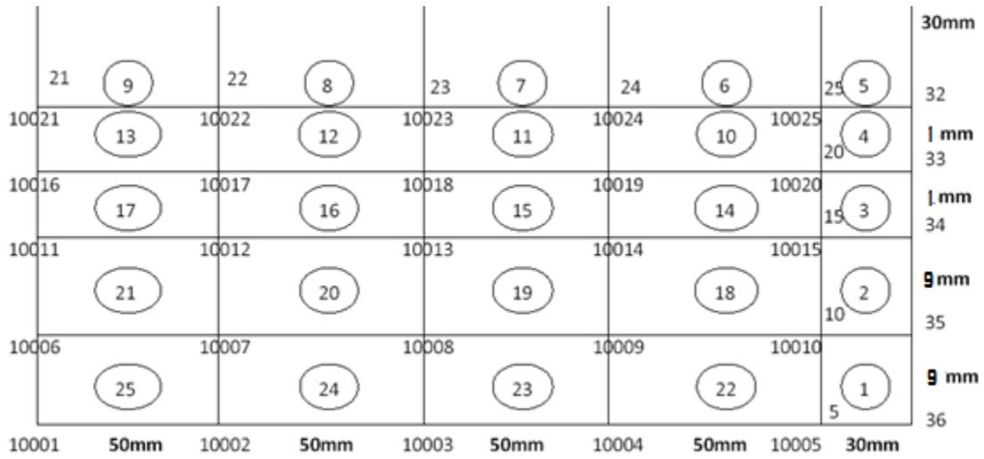
Figure 2 FE model of cross-section of a quarter pultrusion die assembly (not to scale) with foam sandwich pultrudate.
