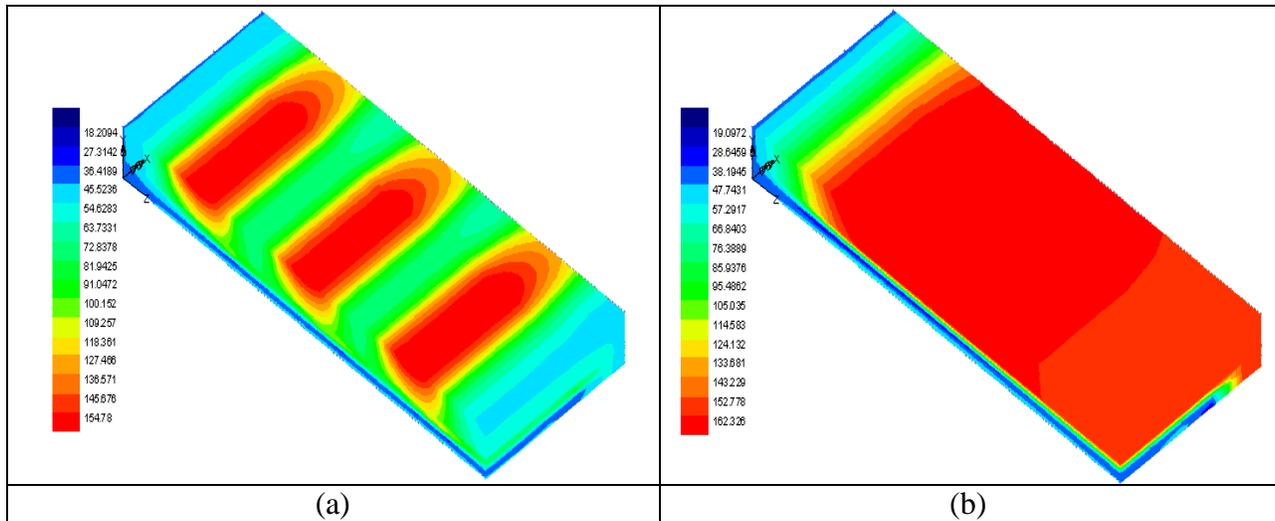
Figure 3, Temperature distribution in modeled pultrusion die assembly at pulling speed of 5mm/s; (a) unsteady state (80 iterations), and (b) steady state (1200 iterations)
