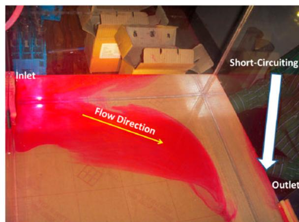
Fig. 3. Rhodamine B tracers at the fifth minute in 50 cm × 50 cm × 50 cm model at 15.5 cm level of water.
