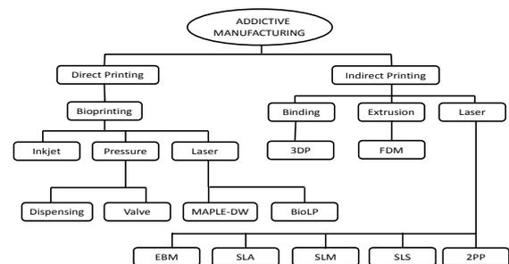
Fig. 3 AM technologies based on the classification mentioned and method to form the structures.
