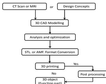
Fig. 2 Brief schematic diagram of product development cycle for 3D printing of bioimplant
