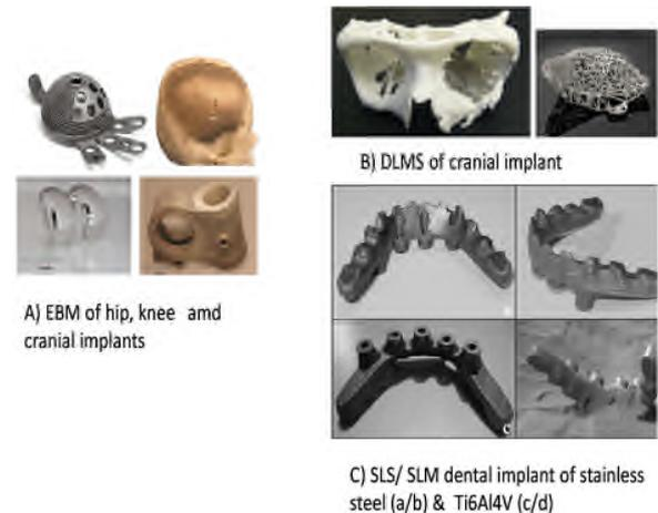
Fig. 6 Metals implants made from A) EBM picture courtesy of Arcam B) DMLS [3] Reproduced by permission of Emeraldinsight and C) SLM/SLS [6] Reproduced by permission of Taylor & Francis
