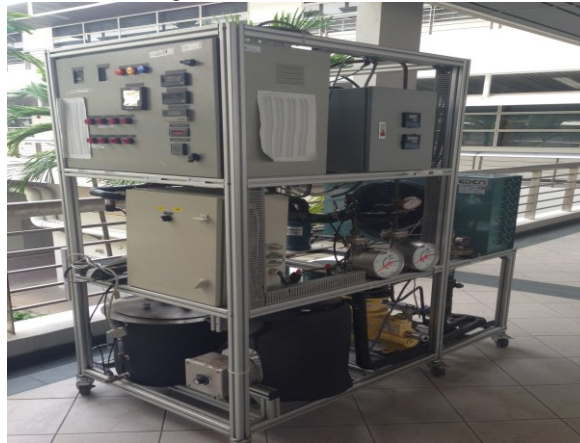
Fig. 1. Photograph of hybrid ejector refrigeration system
