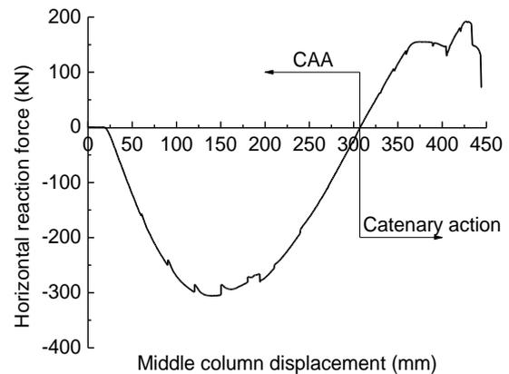
**Fig. 8** Horizontal reaction force-middle joint displacement curve
