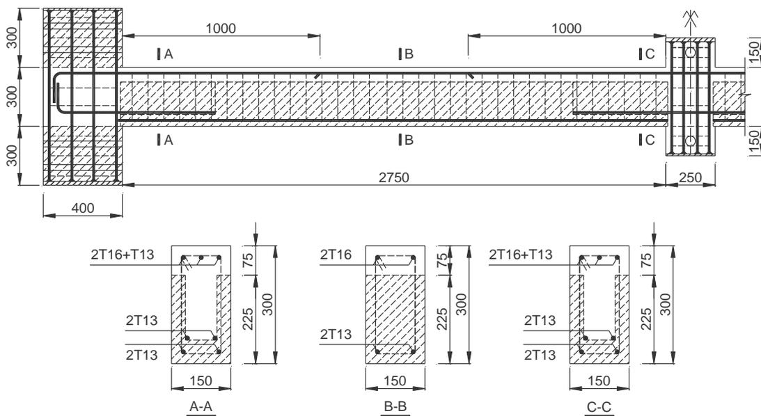
**Fig. 1** Geometry and reinforcement detailing of beam-column sub-assembly
