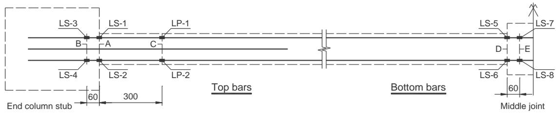
**Fig. 4** Layout of strain gauges on the longitudinal reinforcement of the beam
