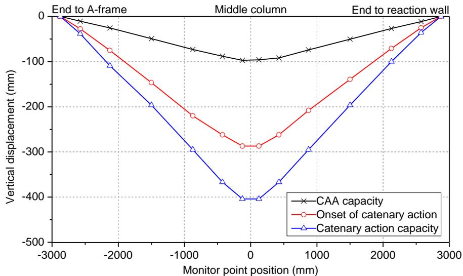
**Fig. 9** Deformed profile of the sub-assembly
