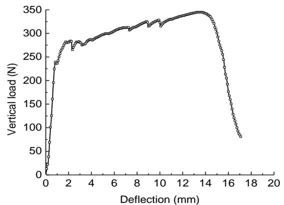
**Fig. 6** Load-deflection curve of ECC plate under four-point bending
