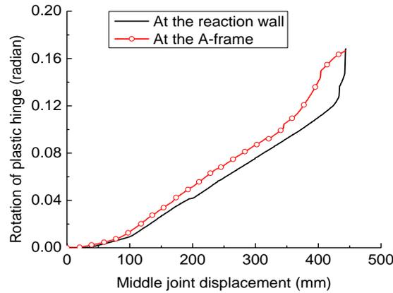
**Fig. 10** Rotation angle of plastic hinges at the end column stubs
