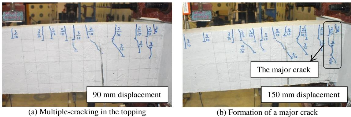
**Fig. 11** Development of multiple cracking in the structural topping
