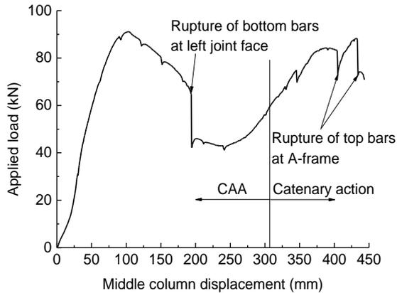
**Fig. 7** Vertical load-middle joint displacement curve
