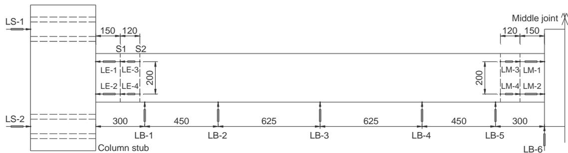
**Fig. 3** Layout of LVDTs on sub-assembly
