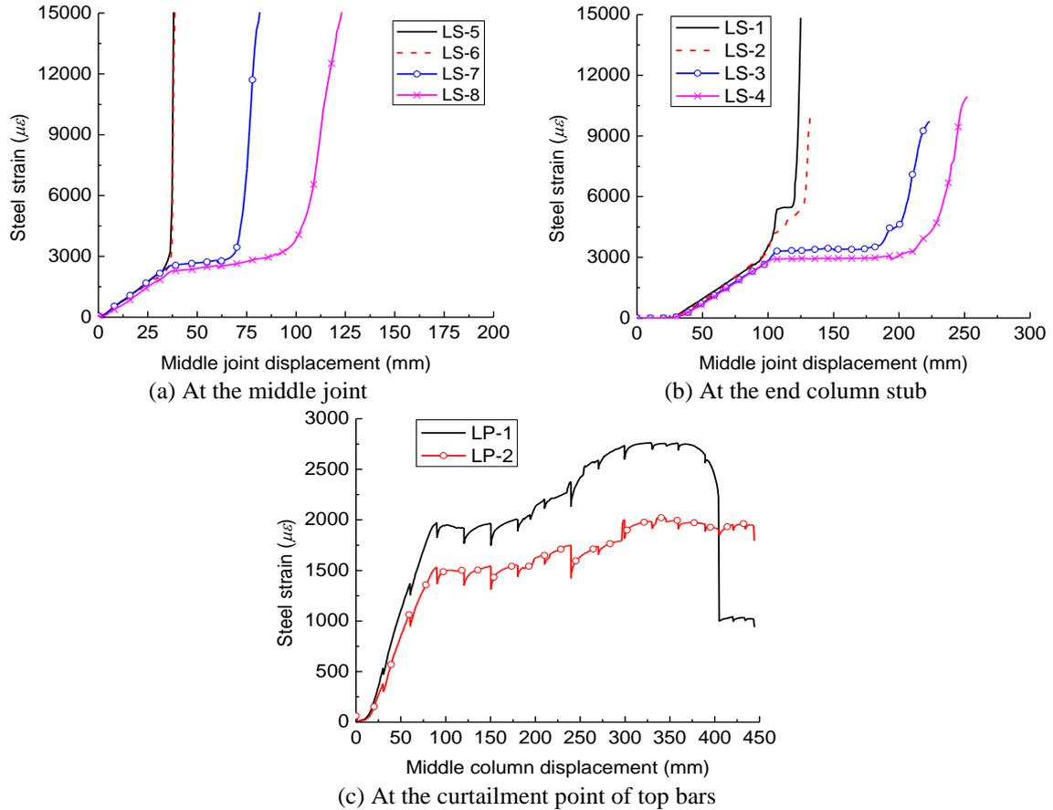
**Fig. 13** Variation of steel strains with middle joint displacement
