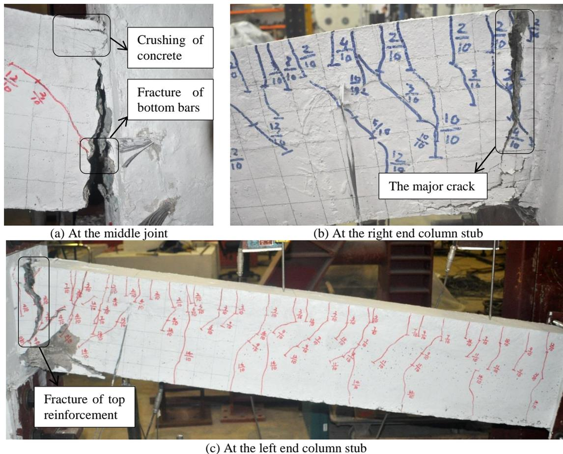
**Fig. 12** Failure modes of the beam-column sub-assembly
