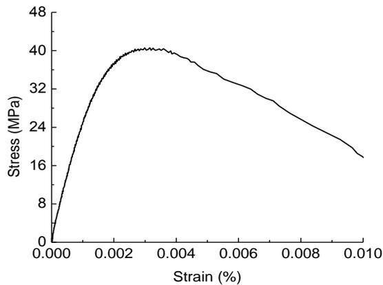
**Fig. 5** Stress-strain relationship of concrete
