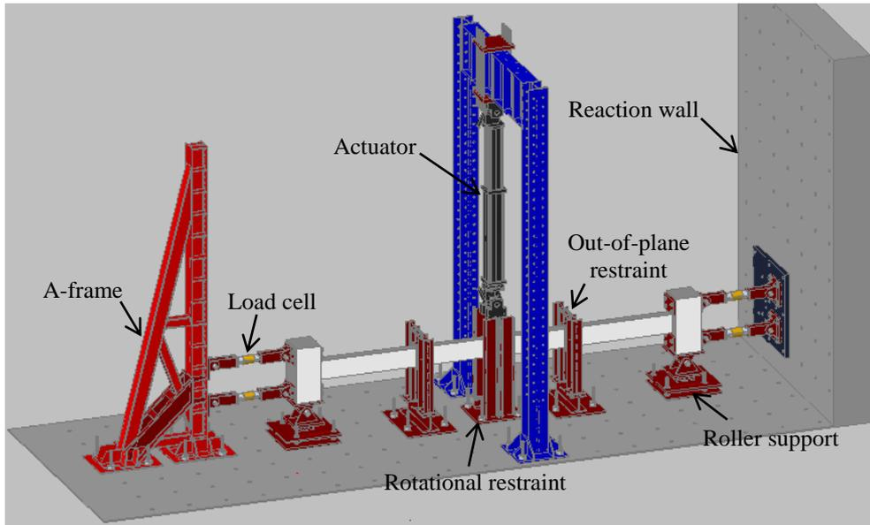
**Fig. 2** Test set-up for beam-column sub-assembly
