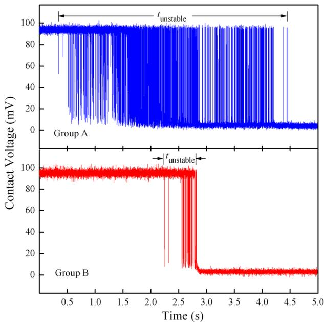
FIG. 1. Contact voltage versus loading time of two typical Au-to-Au contact tests in group A (exposed in MEMS fabrication environment) and group B (reference group, untreated). The duration of the unstable region is denoted as  $t_{unstable}$ .
