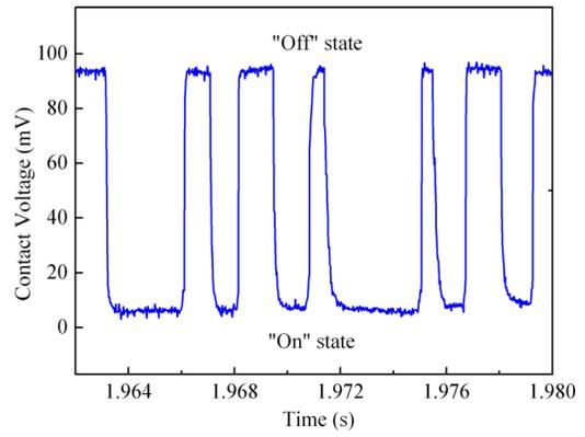
FIG. 2. A close look for a typical contact voltage versus loading time curve measured from a sample in group A. A two-level RTS with “on” and “off” states is shown.
