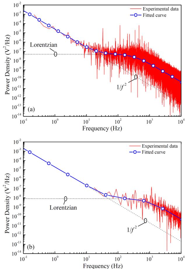
FIG. 3. PSD of the conduction noise in the unstable region for Au-to-Au contacts measured from the samples in (a) group A and (b) group B. The experimental data are fitted by superimposing  $1/f^2$  and Lorentzian components (dashed lines).
