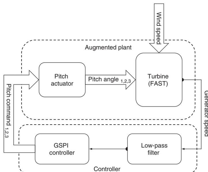
Figure 3: Schematic of gain scheduled PI control (GSPI).
