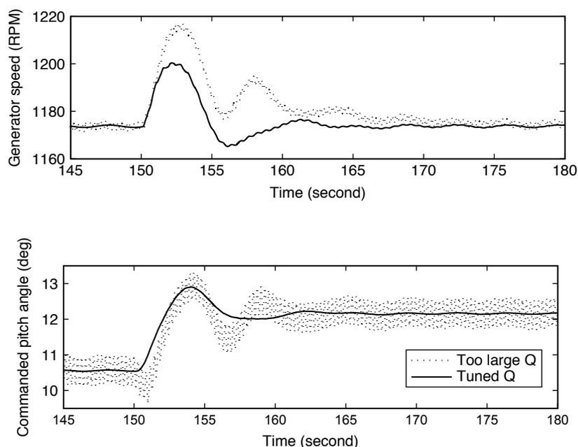
Figure 6: Noisy input and output responses due to large  $Q$ .
