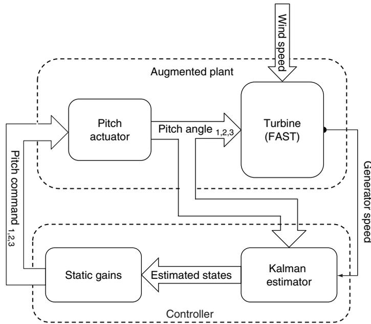
Figure 4: Schematic of stochastic DAC.
