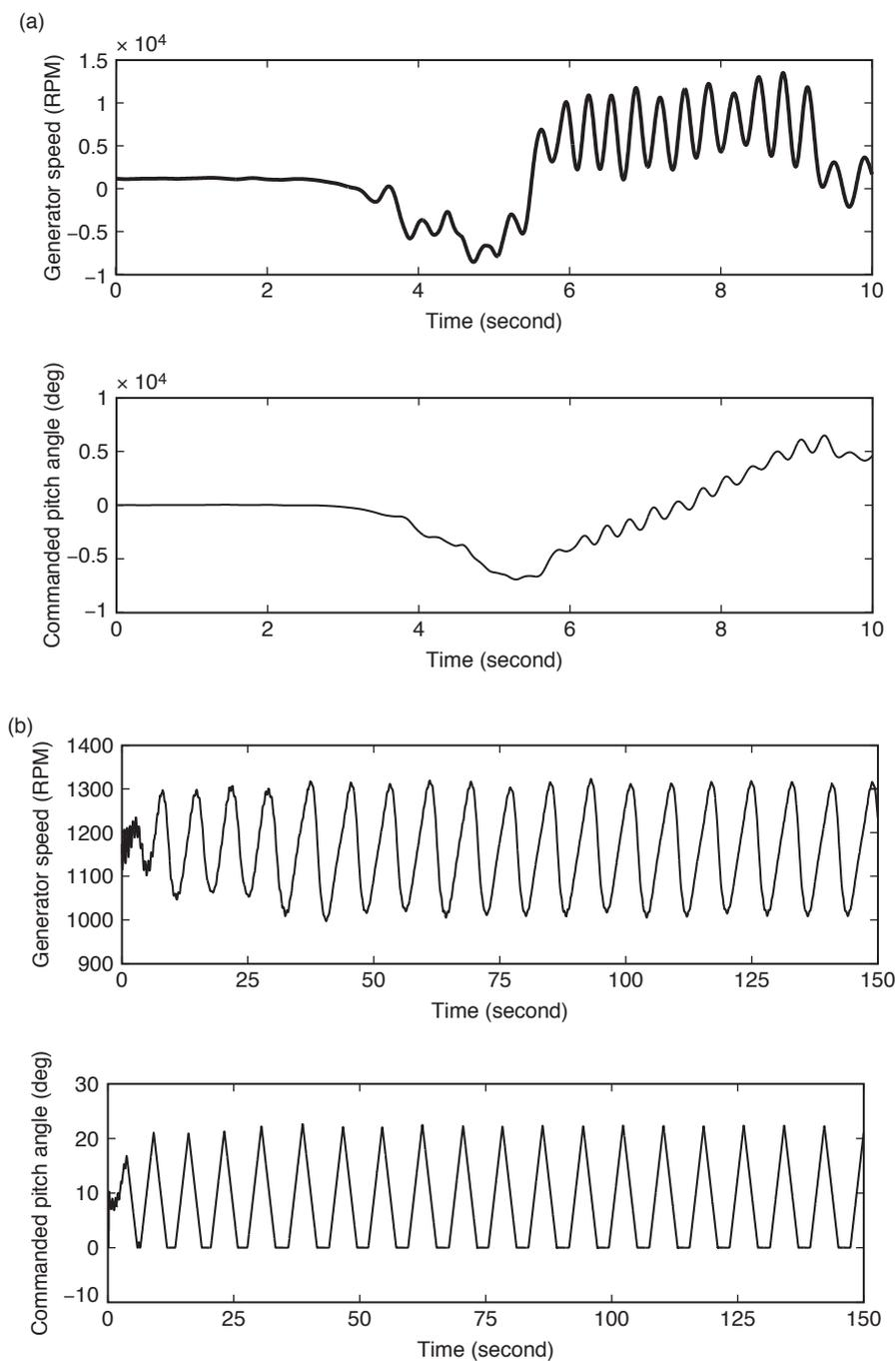
Figure 5: Deterioration in system responses for  $Q = 0$  (a) with an ideal (limitless) pitch actuator, (b) with a pitch actuator having saturation limits.
