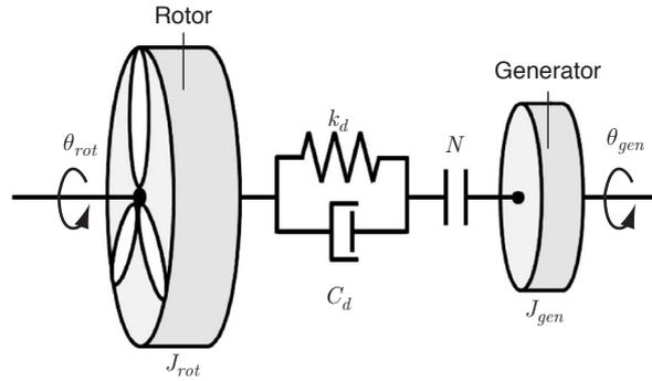
Figure 2: Two-mass model of a wind turbine drivetrain.
