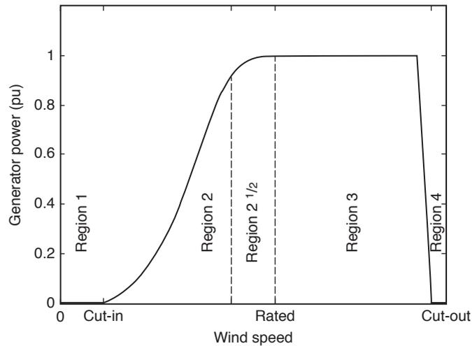
Figure 1: Typical power curve of variable speed variable pitch wind turbine, 1 pu (per unit) power = rated power of the generator.
