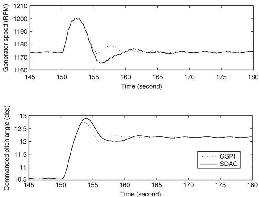
Figure 7: Similar generator speed response GSPI and SDAC after tuning the  $Q$  4.2.1 NREL CART.
