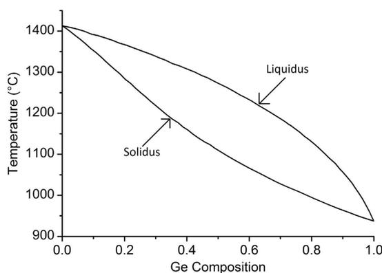
**Figure 2. SiGe phase diagram – adapted from<sup>29</sup>.**
