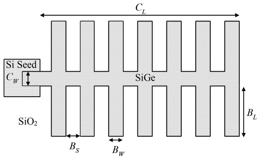
**Figure 3. Schematic of a tree-like structure (plan view).** Dimensions are defined as: centre strip width =  $C_W$ , centre strip length =  $C_L$ , branch width =  $B_W$ , branch length =  $B_L$ , branch separation =  $B_S$ , and number of branches =  $n$ .
