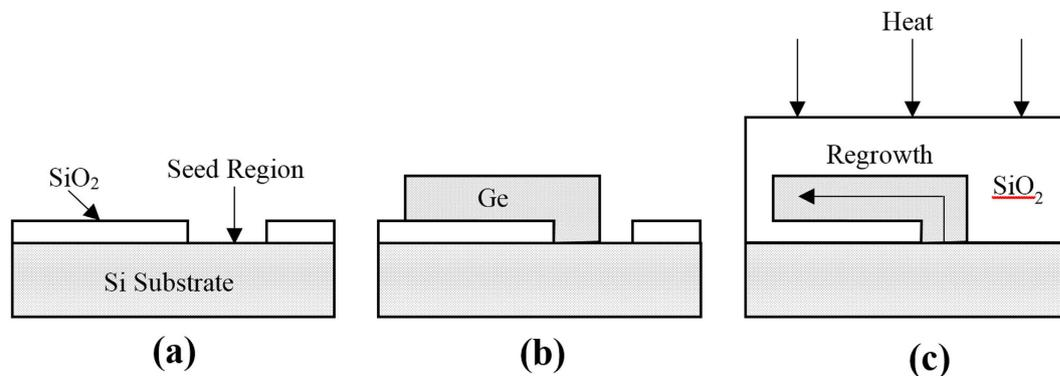
**Figure 1. RMG fabrication process summary (cross-section view).** (a) SiO<sub>2</sub> deposition and patterning, (b) Ge growth and patterning, (c) encapsulation and rapid melting/cooling. Si diffuses from the substrate into the liquid Ge during the melting phase, resulting in solid SiGe formation during cooling.
