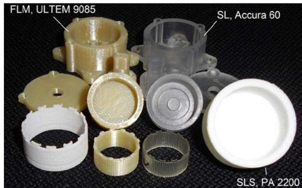
Figure 4: Components of a micro Harmonic Drive gear with tooth module 0.2 mm.
