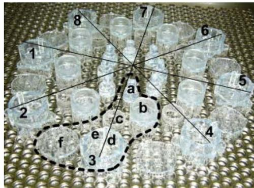
Figure 3. SL Building platform with the components of eight micro Harmonic Drive gears.
