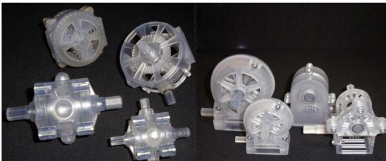
Figure 7: Differential gears and worm gears, SL
