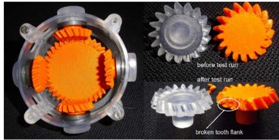
Figure 6: Planetary gear components fabricated by LS and FLM.
