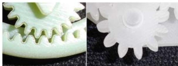
Figure 5: Left gear: module 0.75 fabricated by PJM, right gear: module 1.5 fabricated by MJM.
