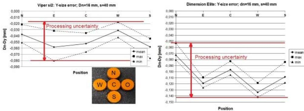
Figure 2. Deviation of Y-diameter from nominal size 16 mm at 5 platform positions.
