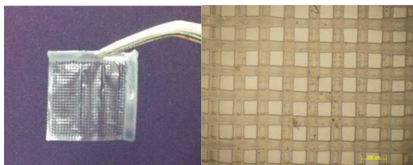
Figure 5: Printed polycaprolactone mesh. Scale bar: 500 \mu\text{m} .
