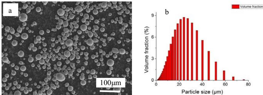
Figure1. (a) SEM image of the powder, (b) The size distribution of the powder
