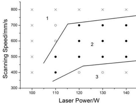
Figure 2. The single track process map. × means the relatively poor tracks, • means the best tracks, and o means the better tracks.
