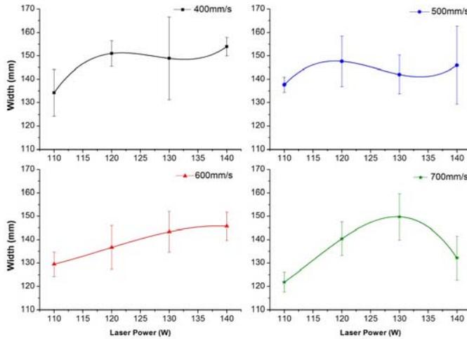
Fig.4 The width of the single track with different laser power and scanning speed
