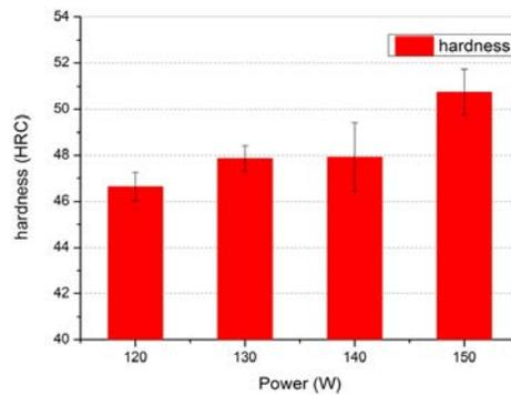
Figure 5. Rockwell hardness results for SLM samples
