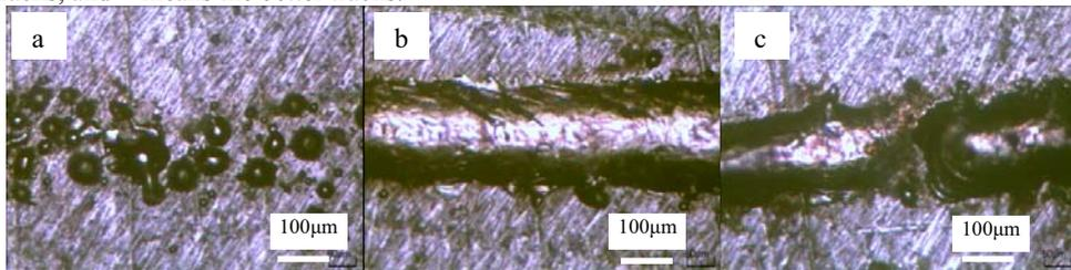
Figure 3. Single track on the steel substrate. (a) P=100W, V=800mm/s; (b) P=140W, V=600mm/s; (c) P=140W, V=400mm/s
