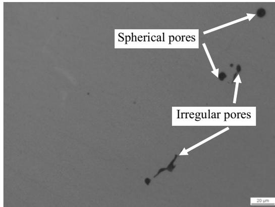
Figure 4. Sample structure of AISI 420 tool steel. Scanning speed=550mm/s, laser power=140W, scanning space=0.07mm, layer thickness=0.02mm.
