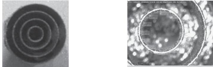
Figure 3. Fabricated specimen and the width of the solidified contour in 500 mm/s and 350W
