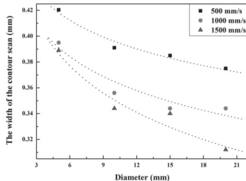
Figure 4. The width of the solidified contour scan with the diameter of circle
