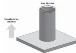
Figure 1. Schematic diagram of SLM process      Figure 2. Shape and manufacturing direction of specimens
