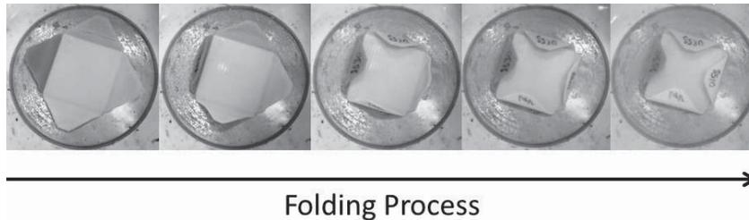
Figure 6. Multi-stage folding square with varying materials at different hinges
