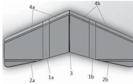
Figure 4. Hinge Location on UAV
