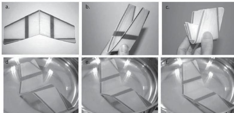
Figure 7. Programming UAV model and recovery of hinges 1a, 1b, 2a and 2b.
