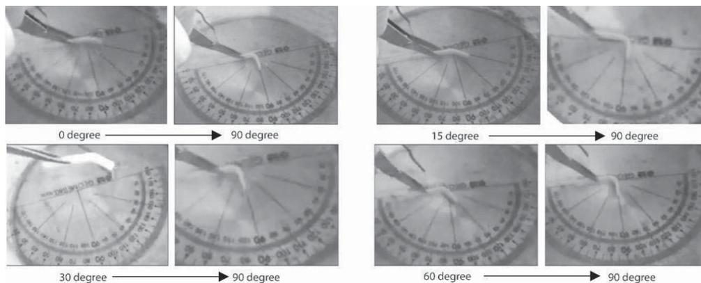
Figure 5. Programmable folding recovers to original 90 degree angle
