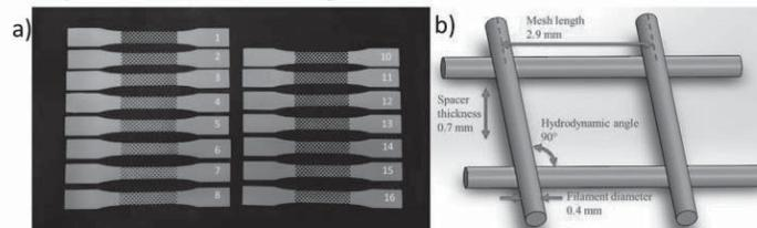
Figure 3: a) EOS SLS printed PP net tensile bars b) Net-typed structure in the tensile bars
