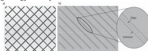
Figure 3: Net-typed structure similar to a feed spacer. a) 3D model b) scan lines of the 3D model at 0.3 mm layer height
