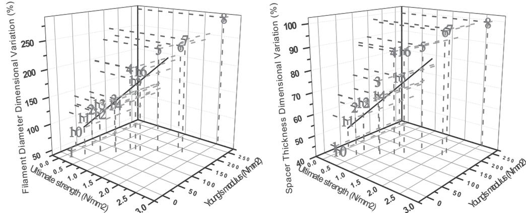
Figure 4: 3D plot of dimensional variation vs ultimate strength vs Young's modulus (left) filament diameter's dimensional variation (right) spacer thickness's dimensional variation
