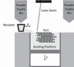
Figure 2: Schematic diagram of the EOSINT P395 SLS machine
