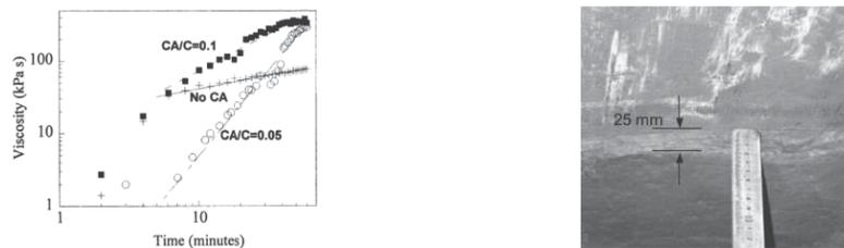
(a) The change in viscosity over time with different proportions of CA and ordinary cement
