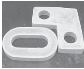
(a) Structures printed by Contour Crafting
