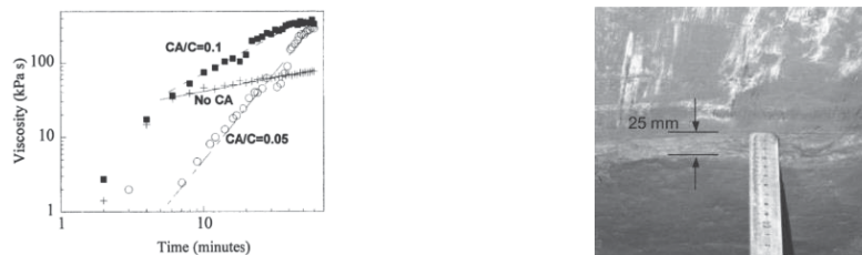
(a) The change in viscosity over time with different proportions of CA and ordinary cement (b) Spray test of shotcrete in the vertical direction
