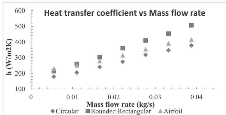
Figure 4. Heat transfer coefficient vs mass flow rate for different heat sinks
