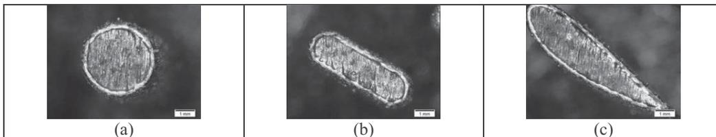
Figure 2. Microscopic view of (a) circular, (b) rectangular rounded and (c) aerofoil fins.
