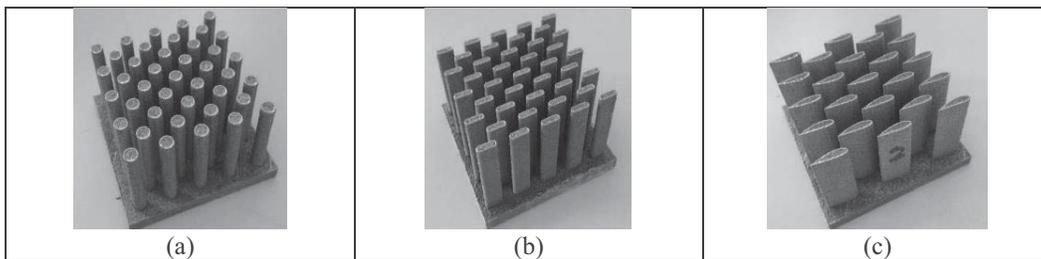
Figure 1. Fabricated heat sinks of (a) circular, (b) rectangular rounded and (c) aerofoil fins.
