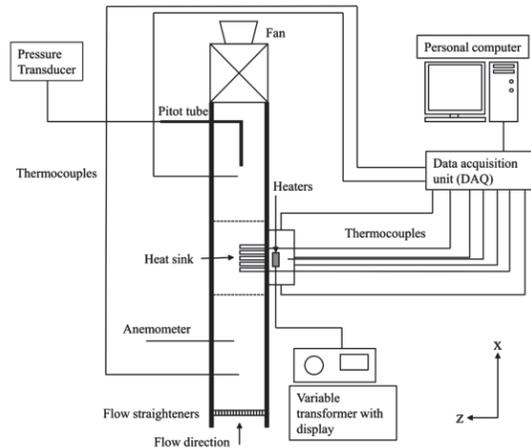
Figure 3. Schematic diagram of setup
