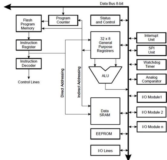
Fig. 3: Block diagram of 8-bit AVR architecture ATmega328P
