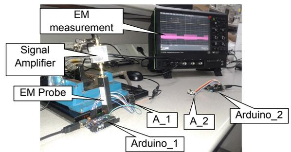
Fig. 6: EM measurement of AES-128 based Arduino implementation
