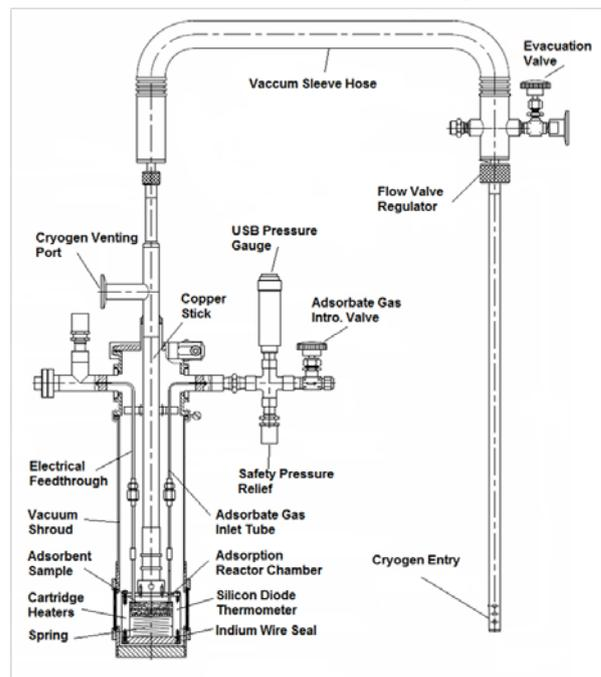
Fig. 2 Schematic diagram of cryogenic adsorption set-up
