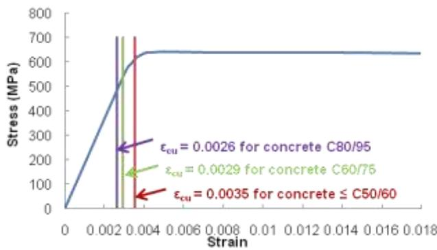
Figure 14. Stress – strain curve of Grade 600 bar
