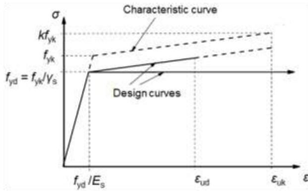
Figure 10. Stress-strain curves for reinforcing steel
