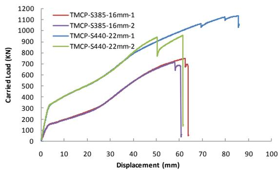
Figure 4. Load-Displacement curves of the TMCP T-stub joints
