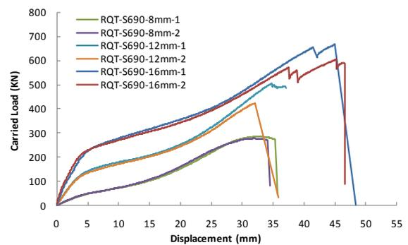
Figure 5. Load-Displacement curves of the RQT T-stub joints
