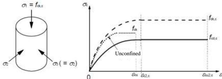
Figure 15. stress-strain relationship for confined concrete
