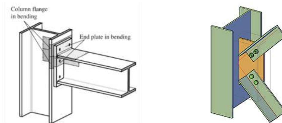
**Figure 2. Beam-column connections (left) and gusset plate connections (right)**
