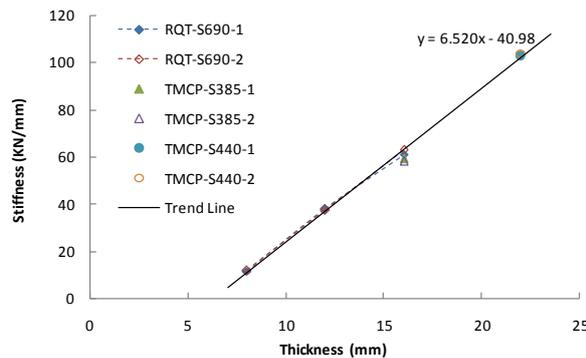
Figure 8. Stiffness of the elastic stage
