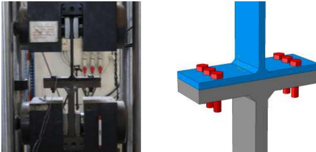
**Figure 3. Tensile test setup (left) and analytical model (right)**
