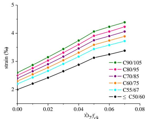
**Figure 16. Increased strain of confined concrete**
