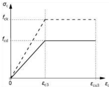
Figure 12 Bi-linear stress-strain relationship
