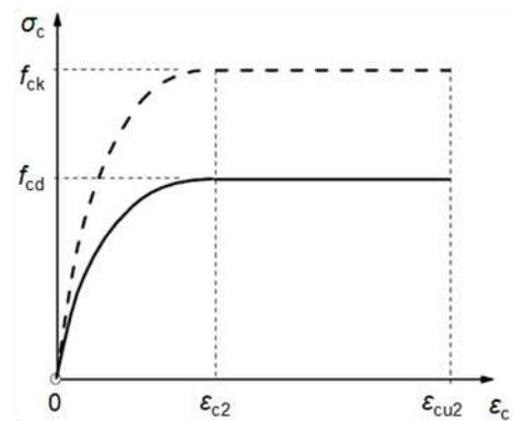
Figure 11. Parabola-rectangular diagram
