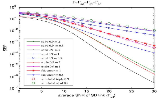
Fig. 1. Performance comparison of triple correlated selection combining technique for NC-BFSK modulation scheme
