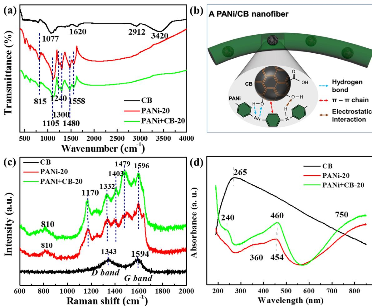
**Fig. 3.** (a) FTIR spectra of CB, PANi-20 and PANi+CB-20. (b) The schematic representation of the formation mechanism of PANi/CB composite. (c) Raman spectra of CB, PANi and PANi/CB electrodeposited on GP. (d) UV-visible spectra of PANi-20 and PANi+CB-20 deposited on Graphite paper.
