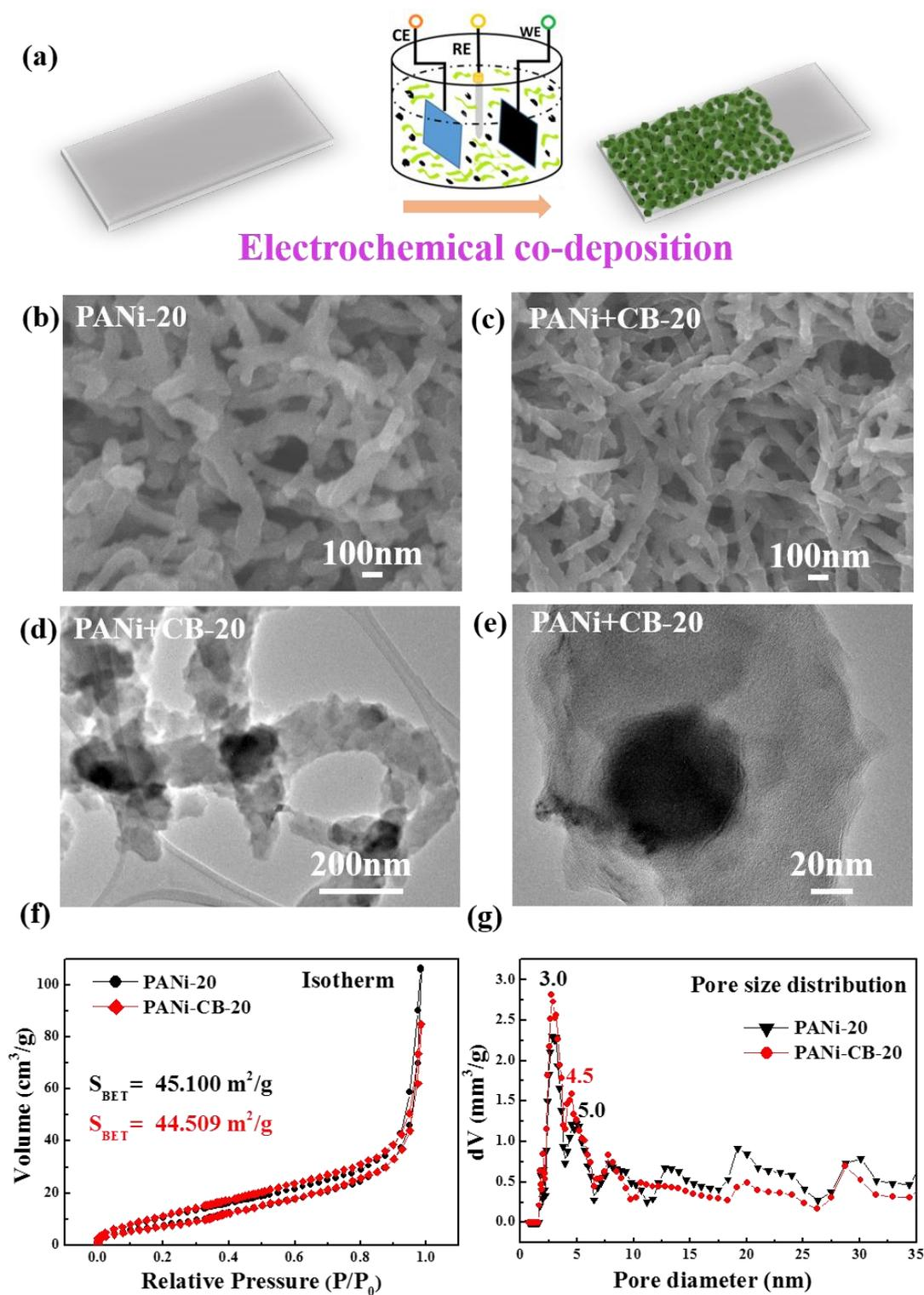
**Fig. 2.** (a) Schematic illustration of the synthesis of PANi based samples deposited on the GP substrate (left). After electrochemical co-deposition (middle), PANi/CB nanofibers are coated on the GP substrate (right). (b), (c) FE-SEM images of PANi-20 and PANi+CB-20, respectively. (d), (e) TEM images of PANi+CB-20 at low and high magnification. (f), (g) The  $\text{N}_2$  adsorption/desorption isotherms and pore size distribution (PSD) curves of PANi-20 and PANi+CB-20.
