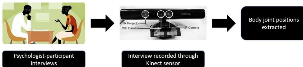
Fig. 1. The video recording hardware and joint position extraction system.
