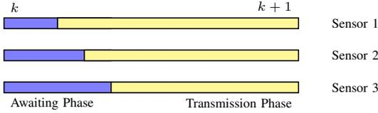
**Fig. 1:** Illustration of the awaiting phase and transmission phase for three sensors between time  $k$  and  $k + 1$ .
