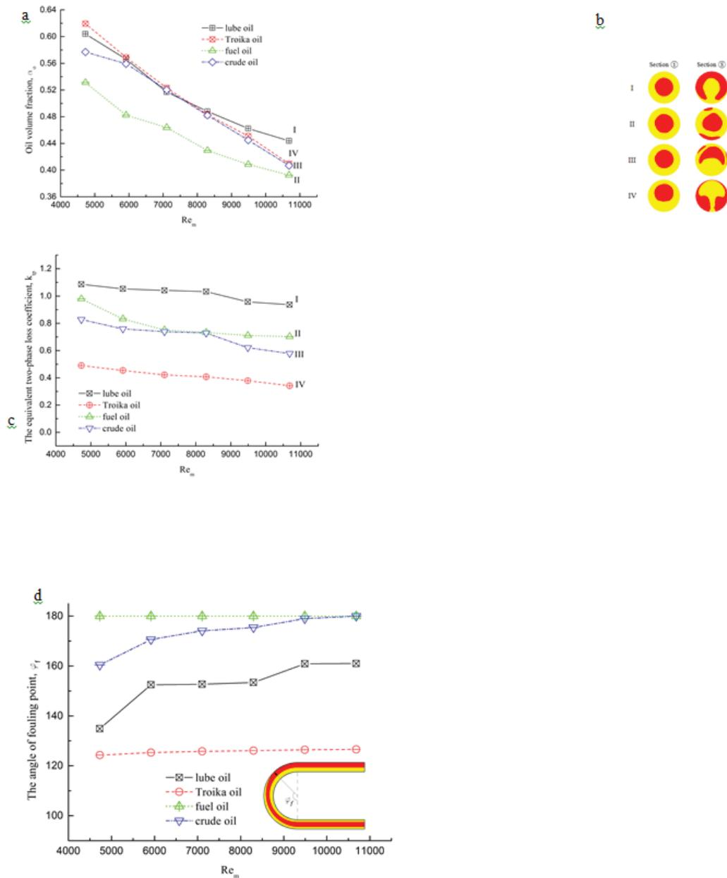
Fig. 6 The influence of oil property. (a) Variation of  $\alpha_o$  with different oil property; (b) the oil phase fraction contours at points of I-IV; (c) variation of  $k_{tp}$  with different oil property; (d) variation of  $\varphi_f$  with different oil property.
