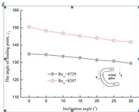
Fig. 7 The influence of inclination angle. (a) Variation of  $\alpha_o$  with different inclination angle; (b) variation of  $k_p$  with different inclination angle; (c) the phase fraction contours at points of I-IV; (d) variation of  $\varphi_f$  with different inclination angles.
