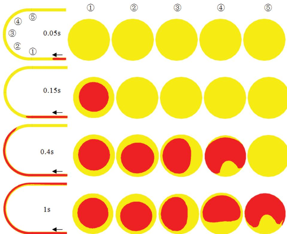
Fig. 4 Development of core flow at section 1- section 5 during upflow through U bend;  $v_{so} = 0.6$  m/s,  $v_{sw} = 0.4$  m/s; oil, water.
