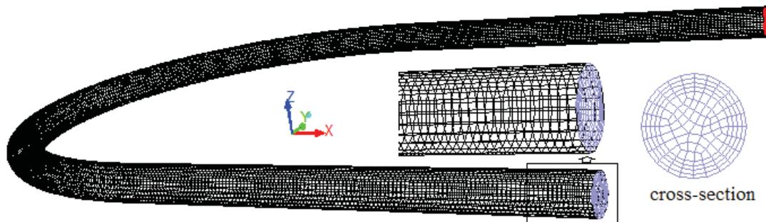
Fig. 2 The meshed geometry.
