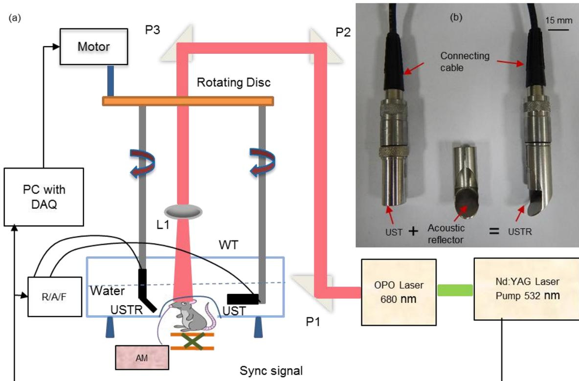
Fig. 1 (a) Schematic diagram of the PAT set up. P1, P2, P3: coated prisms; DAQ: Data Acquisition card; R/A/F: Receiver/Amplifier/Filter; UST: Ultrasound Transducer; USTR: Ultrasound transducer with reflector; WT: Water tank; L1: Plano concave lens; AM: Anesthetizing Machine. (b) Image of conventional UST and acoustic reflector attached to the conventional UST.
