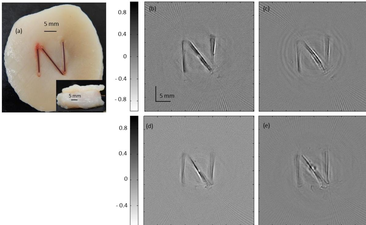
Fig. 2 (a) ‘N’ shaped blood vessel phantom embedded inside chicken breast tissue (inset: one more layer of 5 mm thick chicken breast tissue placed on top). (b), (c) reconstructed PA images obtained using flat UST and flat USTR respectively. (d), (e) reconstructed PA images obtained using focused UST and focused USTR respectively.
