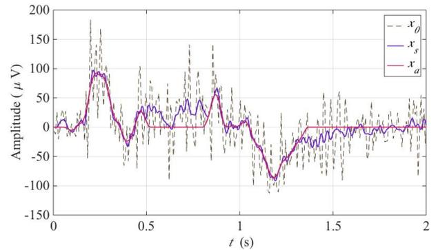
Fig. 1. Examples of the construction of artifact signal.  $x_0$  is the raw data,  $x_s$  is the smoothen data, and  $x_a$  is the constructed artifact, which are all zeros except for the segments containing the peaks within the certain peak amplitude range.
