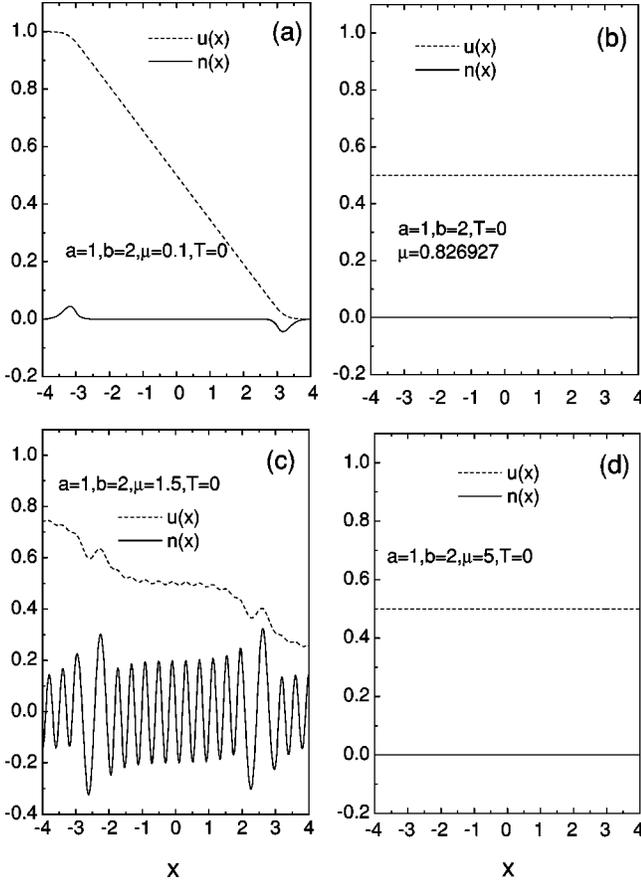
FIG. 2. The distribution of internal potential (dashed line) and charge density (solid line) for  $a=1$ ,  $b=2$ , and  $T=0$ . (a) The small-transmission case,  $\mu=0.7$ , (b) The resonant case,  $\mu=0.26927$ , (c)  $\mu=1.5$ , above the barriers, and (d)  $\mu=5$ , well above the barrier height.
