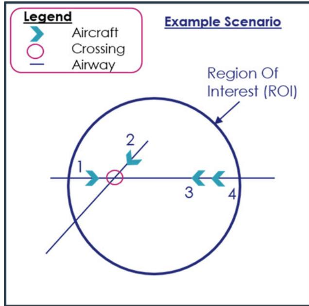
Figure 3. Example scenario - a set of four aircraft registered in a radar at a particular time frame.
