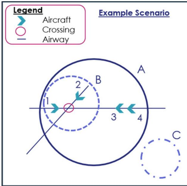
Figure 4. Example scenario - a set of four aircraft having three different ROIs at a particular time frame.
