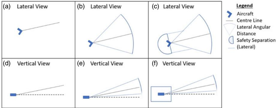
Figure 1. (a–f) Establishment of an aircraft's conflict shape movement.
