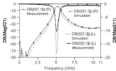
Fig. 6. Comparison of the theory and experiment results of the proposed filter.
