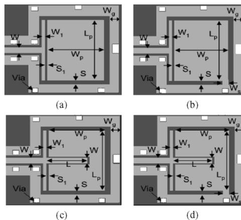
Fig. 2. Ground ring guarded patch resonators (a) rectangular (b) rectangular with shunt (c) “U” shape (d) “U” shape with shunt: Black = Substrate. Grey = metal.
