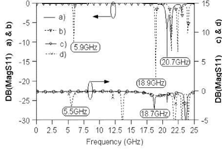
Fig. 3. Frequency response of the resonators in Fig. 2:  $W_1 = 50 \mu\text{m}$ ,  $W_p = 2 \text{ mm}$ ,  $L_p = 2.28 \text{ mm}$ ,  $W_s = 0.2 \text{ mm}$ ,  $S = 0.15 \text{ mm}$ ,  $W_1 = 0.1 \text{ mm}$ ,  $S_1 = 0.1 \text{ mm}$ ,  $W_g = 0.3 \text{ mm}$ ,  $L = 1.8 \text{ mm}$ ,  $W = 0.2 \text{ mm}$ ,  $S_{in} = 0.12 \text{ mm}$ .
