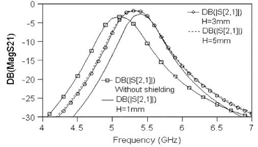
Fig. 5. Comparison of shielding effect on ring guarded shunt patch filter.
