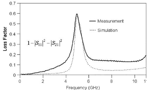
Fig. 7. Comparison of the theory and experiment loss factor of the filter.
