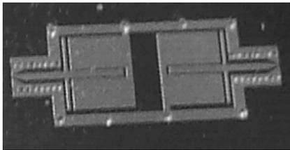
Fig. 8. Enlarged photo of the proposed filter in Fig. 1 Size: 8.7 mm  $\times$  2.9 mm.
