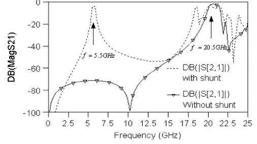
Fig. 4. Comparison between Fig. 2(a) and (b) type filters  $A = 5 \text{ mm}$ ,  $B = 7.9 \text{ mm}$ ,  $H = 5 \text{ mm}$ ,  $S_1 = 0.05 \text{ mm}$ ,  $G = 1 \text{ mm}$ , other parameters (see Fig. 3).
