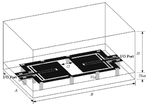
Fig. 1. Perspective view of ring guarded shunt patch filter ■ metal.
