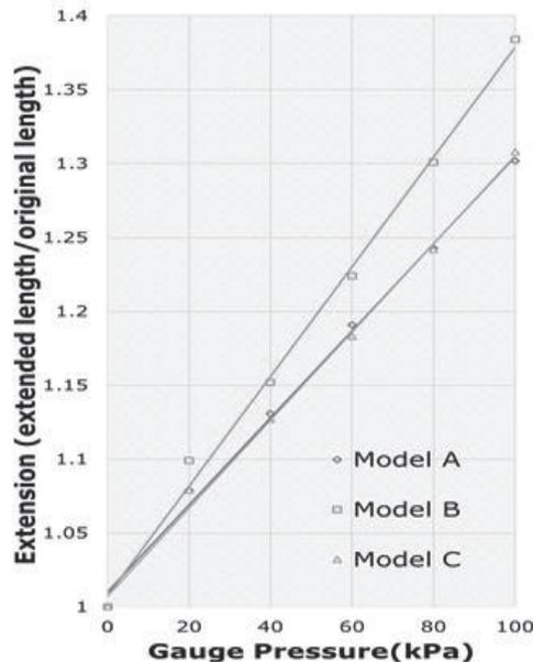
Figure 2. The extension of the actuator at different gauge pressure for three design actuator configurations.
