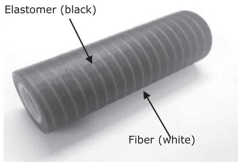
Figure 1. Fiber reinforced soft composites: fiber (white) winding around the elastomer material (black)
