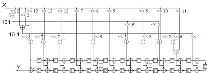
Fig. 8. Symmetric filter with common subexpressions 101 and 10I.
