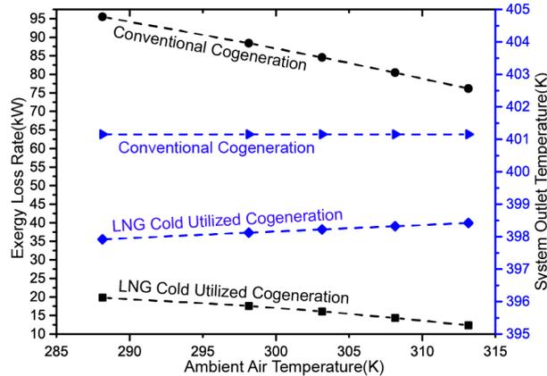
Fig.4: Exergy loss and outlet temperature values of both micro-cogeneration systems.
