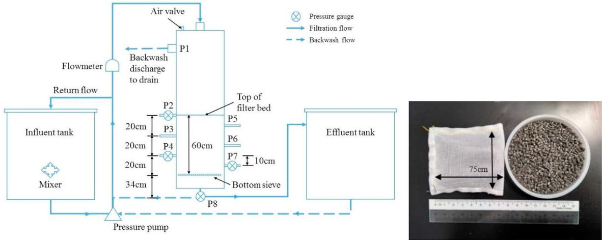
Fig 1. (Left) Schematic representation of lab-scale rapid pressure filter setup; (Right) A typical representation of the packed RPCs.
