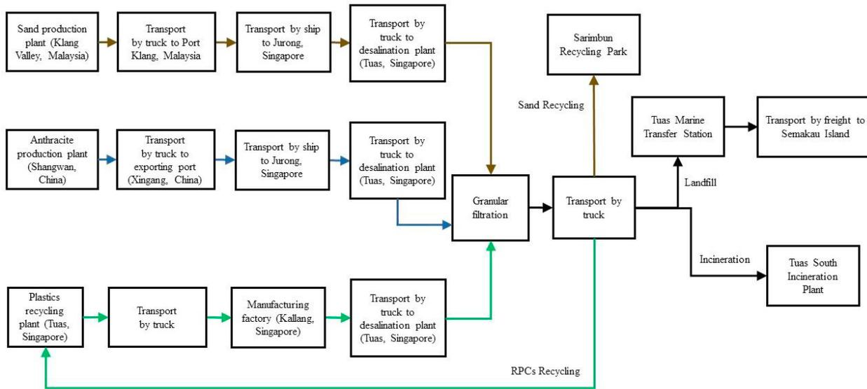
Fig 2. System boundary for DM and PC configurations and Processes involved in the LCA study.
