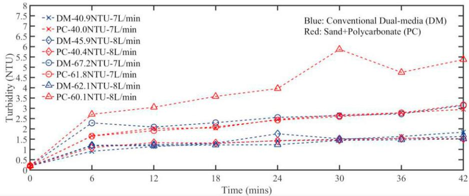
Fig 3. Turbidity at P8 (effluent) for rapid filtering of 20µm monodisperse suspensions.
