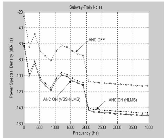
Fig.3 Spectrum showing noise reduction using NLMS and VSS-NLMS algorithms (Subway train noise)
