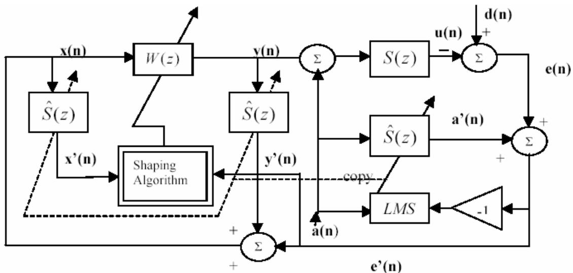
Fig.2 Block diagram of a generic combined audio and feedback ANC system
