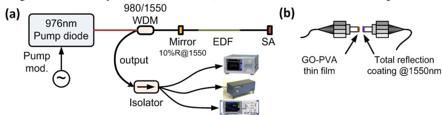
**Fig. 2.** (a) Laser design with linear cavity; (b) Placement of GO-PVA and CNT-PVA thin film saturable absorbers.
