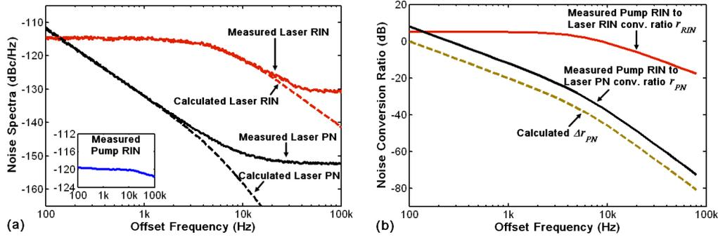
**Fig.4.** (a) Noise spectra of the SESAM laser. Inset: Pump RIN spectrum; (b) Measured noise conversion ratios and calculated excess phase noise conversion  $\Delta r_{PN}$  due to the slow saturable absorber effect
