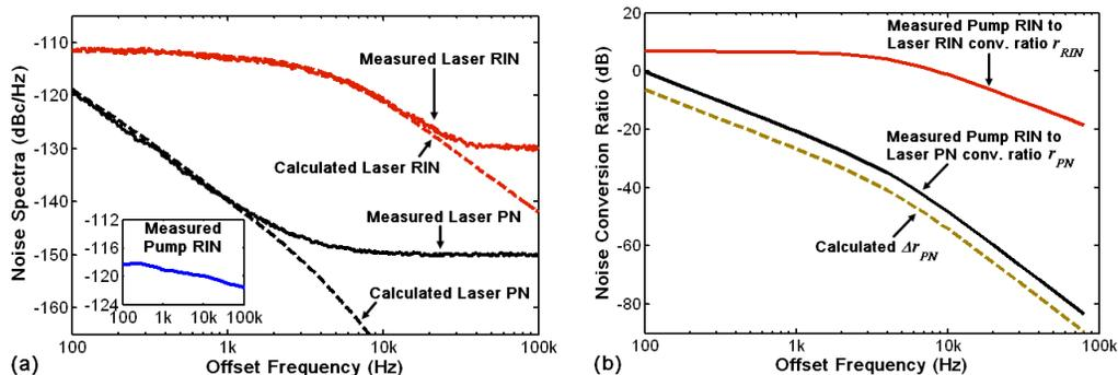
**Fig.3.** (a) Noise spectra of the GO laser. Inset: Pump RIN spectrum; (b) Measured noise conversion ratios and calculated excess phase noise conversion  $\Delta r_{PN}$  due to the slow saturable absorber effect.
