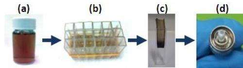
**Fig. 1.** Preparation of GO-PVA and CNT-PVA thin film SAs (a) GO and CNT dispersed solution; (b) polystyrene cells filled with solutions; (c) thin film stripped off the cell wall after heating and evaporation process; (d) small piece of thin film SA on a fiber end
