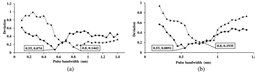
Fig.4 Relationship between 2<sup>nd</sup> order differentiator deviation and the 3-dB bandwidth of the input pulse, the input pulse central wavelength is (a) 1550 nm (spacing between two heated regions is 3 elements for the dot and 6 for the triangle) (b) 1549nm (spacing is 4 and 7 elements)
