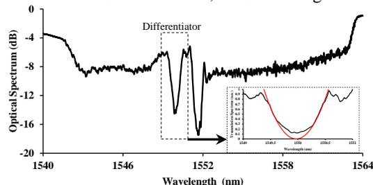
Fig.2: Transmission spectrum of the LCFBG and the local transmission spectrum (solid curve) compares with the ideal transmission function of the 2nd order differentiator (red curve).
