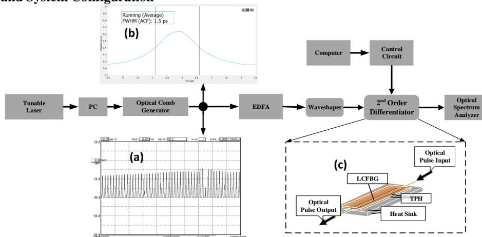
Fig. 1: Experimental setup of the 2nd order optical temporal differentiator, (a) optical comb generator output spectrum, (b) optical comb generator time-domain pulse waveform, (c) construction of the second-order differentiator
