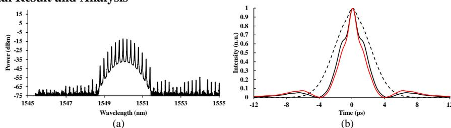
Fig.3 (a) Optical spectrum of the input signal and (b) Input and output time-domain waveform of the 2<sup>nd</sup> order optical differentiator. Input Gaussian-like pulse (dashed black curve), experimental (solid black curve) and ideal (red curve) output waveform of the 2<sup>nd</sup> order differentiator.
