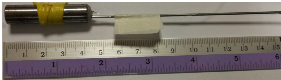
Figure 2. Fabricated FBG Sensor
