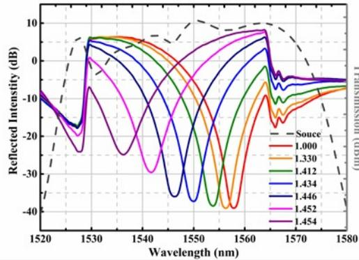
Figure 3 Transmission spectrum of BBS and reflection spectral evolution of the refractometer under various refractive indices.
