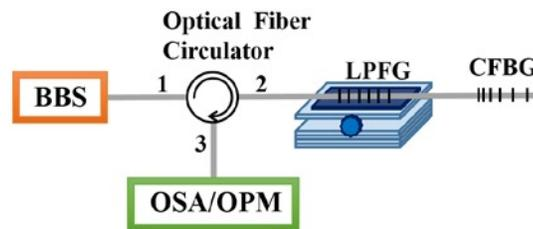
Figure 2 Experimental setup for RI measurement.
