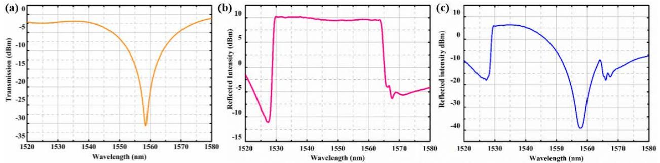
Figure 1 (a) Transmission spectrum of the LPG; (b) Reflection spectrum of the CFBG. (c) Reflection spectrum of the LPG cascaded with the CFBG.
