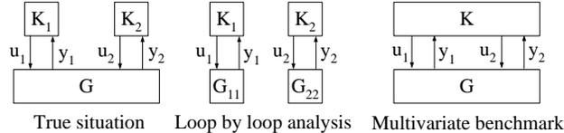
Fig. 1. Insufficiency of available Minimum Variance based benchmarks for performance assessment of systems under decentralized control
