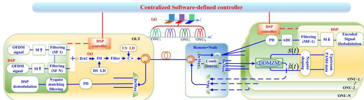
Fig. 1. Bidirectional SSB modulation for WDM-PON with source-free ONUs.
