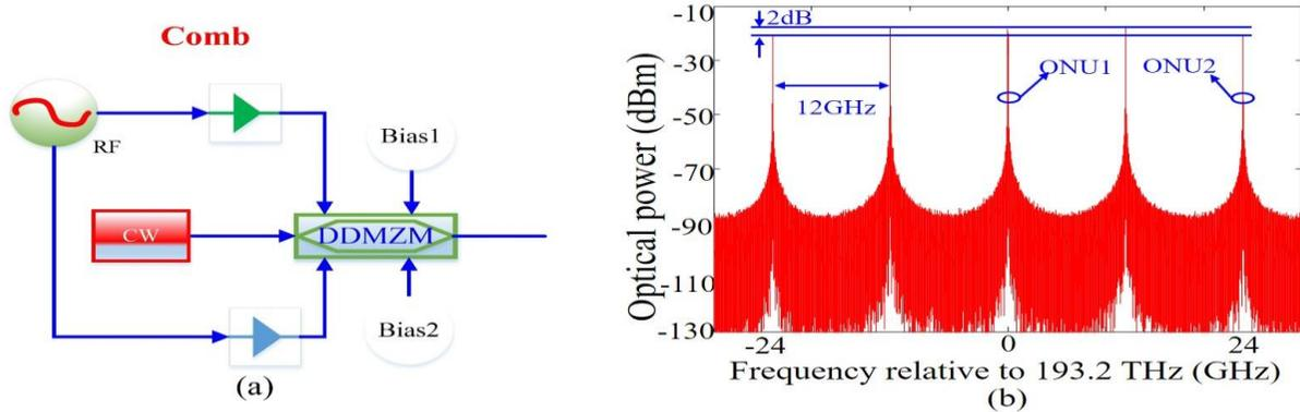
Fig. 2. (a) The schematic diagram of generating OFC with DDMZM; (b) the generated OFC with a frequency separation of 12 GHz.
