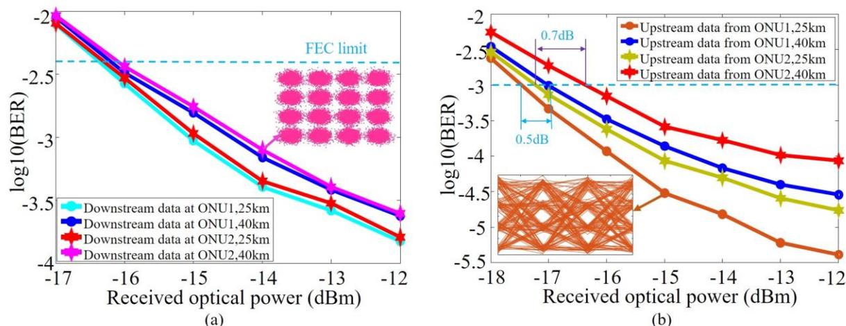
Fig.4. BER performance versus the received optical power; (a) for downstream signal, (b) for upstream signal.
