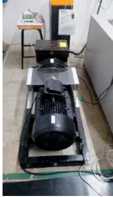
Fig. 4. Image of 13.5kVA, 4 pole, Marelli Generator the synchronous generator in W or kW and \bar{c} represents the no-load speed of the synchronous generator in rpm.
