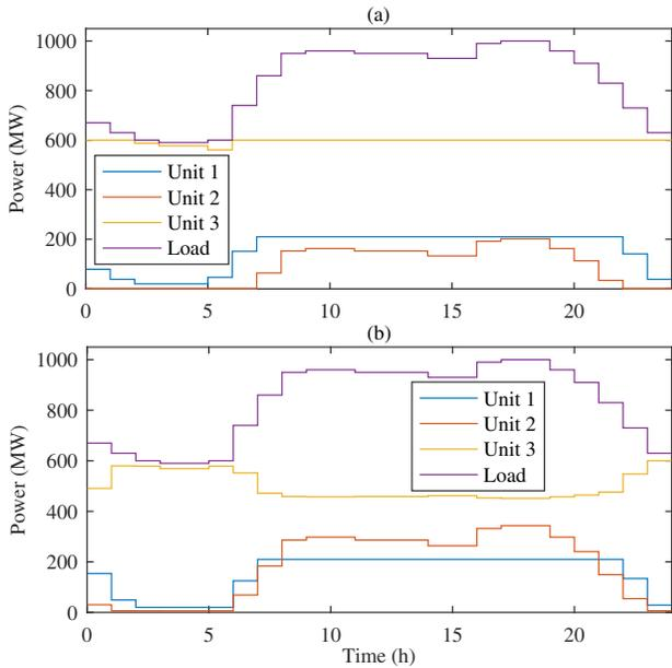
Figure 2. Power dispatch schedule for (a) the HTG and (b) the ACG.
