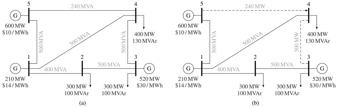
Figure 1. Single-line diagrams of the adapted PJM system (cf. [22]), where (a) is the original ACG and (b) is the HTG obtained by upgrading AC line 3–4 and 5–4 to HVDC. Note that (unidirectional) HVDC lines are represented by a (directional) dashed line [4, Fig. 1].
