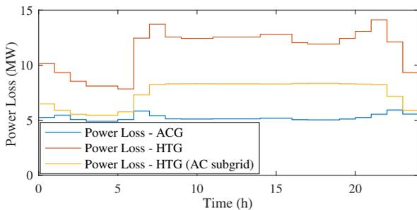
Figure 3. Losses of the ACG and HTG (with and without HVDC losses).
