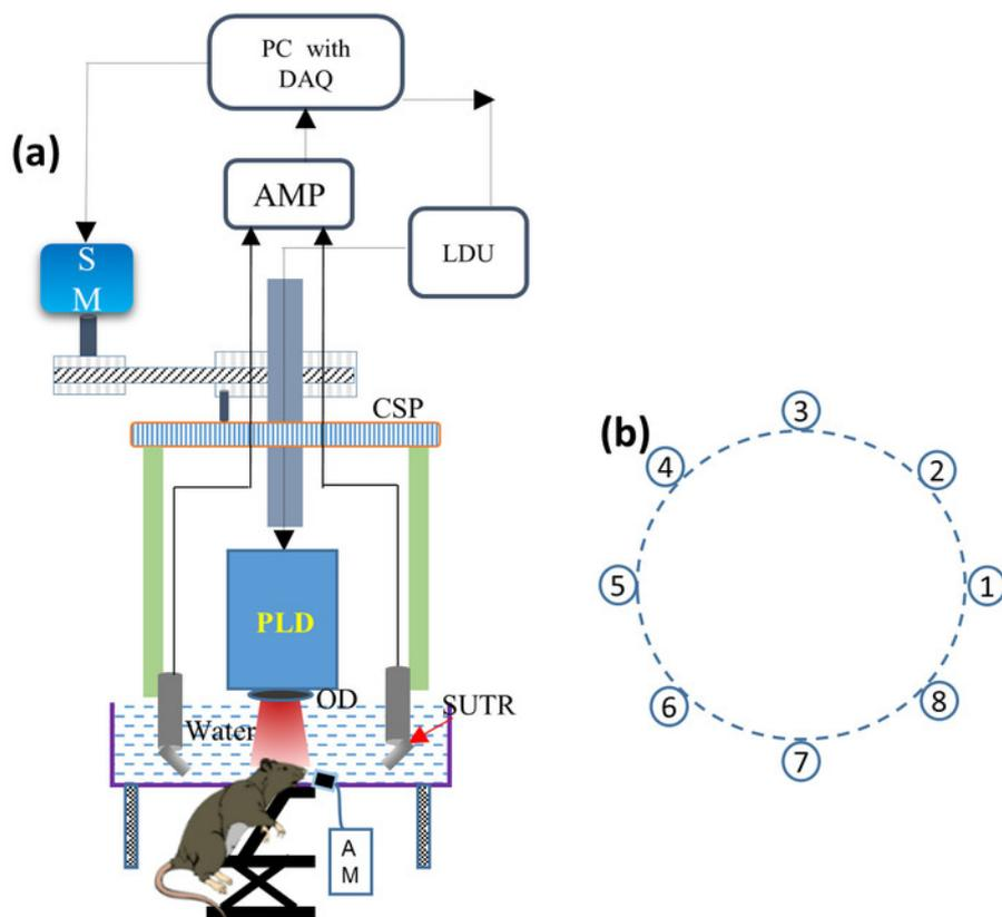
**Figure 1: Schematic of the desktop PLD-PAT system.** (A) Schematic of the desktop PLD-PAT set up. PLD: pulsed laser diode, OD: optical diffuser, SUTR: acoustic reflector based single-element ultrasound transducer, AM: anesthesia machine, CSP: circular scanning plate, SM: stepper motor, LDU: laser driving unit, AMP: amplifier, DAQ: data acquisition card. (B) Circular arrangement of eight SUTRs around the scanning center. [Please click here to view a larger version of this figure.](#)
