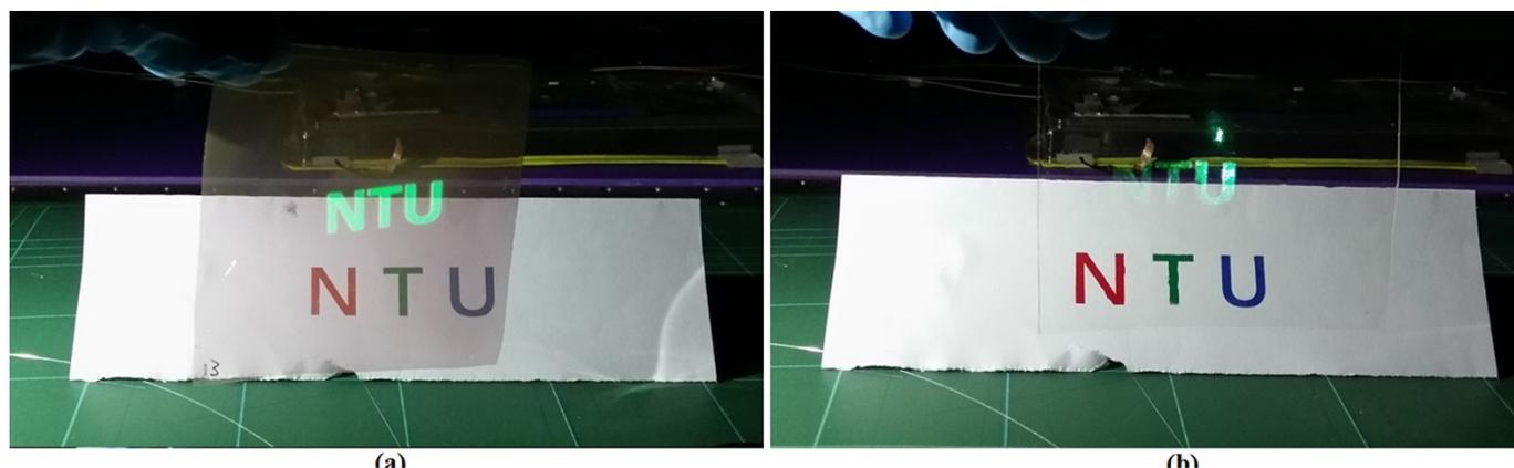
**Fig. 6** Demonstration of the transparent nanoparticle-dispersed PVA film which selectively scatters green light (a). A pure PVA film without nanoparticle is shown for comparison (b). The images were projected by a laser projector (SONY MP-CL1A). The images of (a) and (b) are captured with the same lighting and exposure conditions, and the photographs are not edited.
