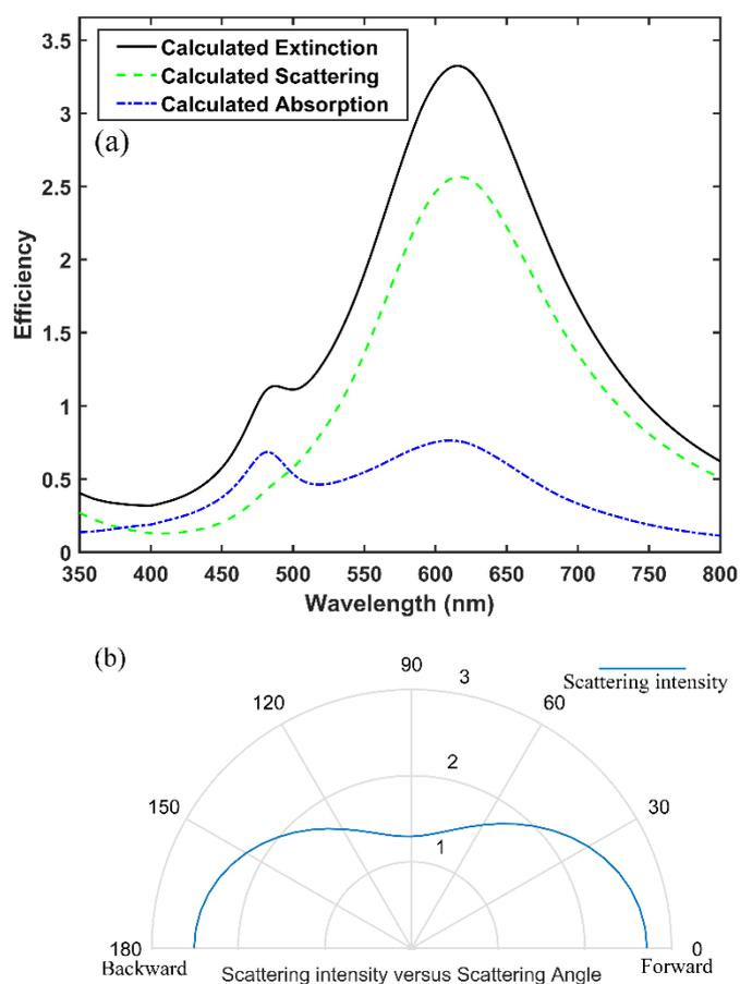
**Fig. 7** (a) Efficiency (defined by  $(cross\ section)/\pi a^2$ , where  $a = 76.5$  nm) for extinction, scattering and absorption, calculated by Mie’s theory for the
