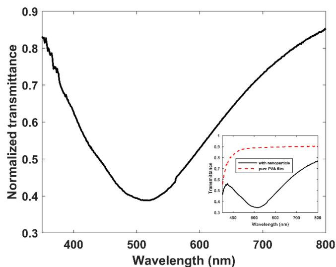
**Fig. 4** Transmittance of the  $Ag@TiO_2$ -dispersed PVA film normalized to the pure PVA film, having an average value of 60.38%. The inset shows the comparison of the transmittance between the  $Ag@TiO_2$ -dispersed PVA film and the pure PVA film.
