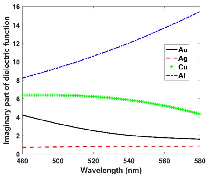
Fig. 1 Imaginary part of dielectric functions ( $\varepsilon_2(\omega)$ ) around the 530 nm for Au, Ag, Cu and Al. Optical constants are taken from reference.<sup>16</sup>
