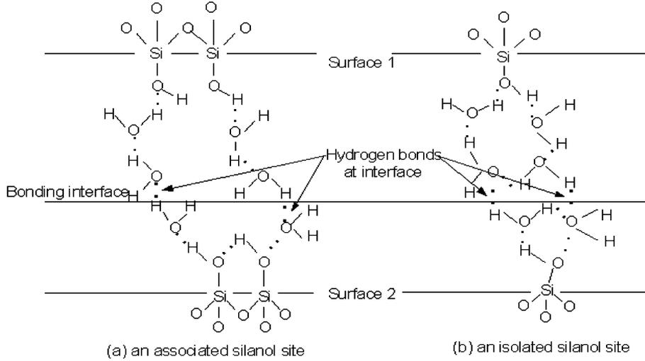
Fig. 2. Postulated interface chemical structures of hydrophilic Si/Si pairs immediately after RT contacting (a) at an associated silanol site and (b) at an isolated silanol site (reproduced from [9, Fig. 4.27] for ease of discussion).
