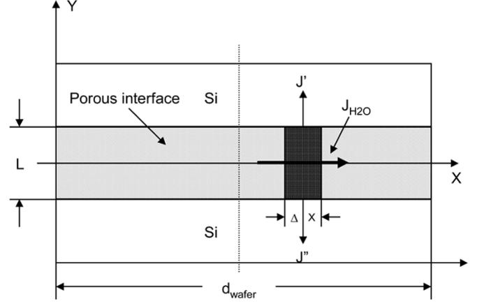
Fig. 1. Schematic of the proposed diffusion model of water at bonded interface.
