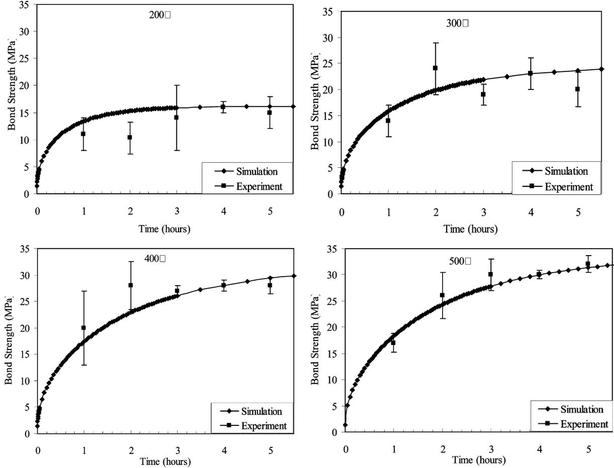
Fig. 3. Comparison between vacuum wafer bond strength of experiments and that of simulation after different annealing processes.
