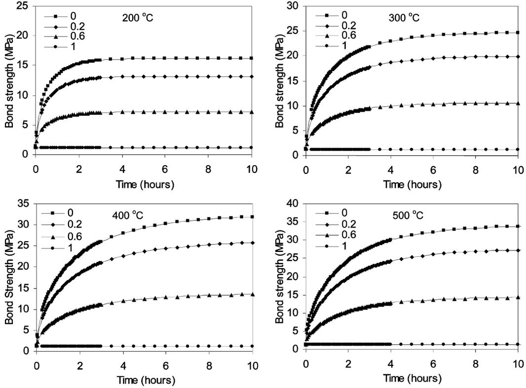
Fig. 4. Simulation results of the effect of vacuum level on bond strength.
