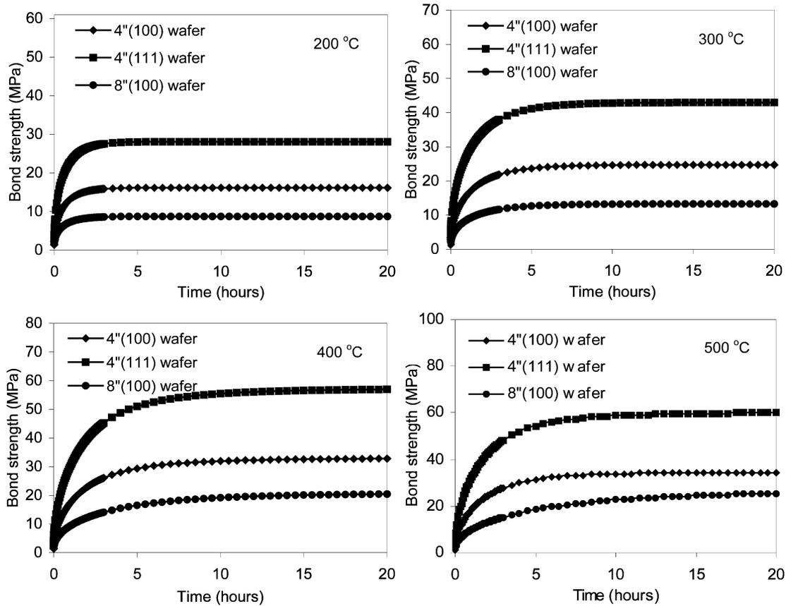
Fig. 5. Effect of wafer dimension on bond strength.
