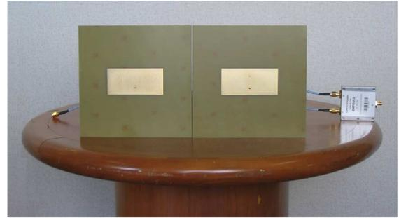
Fig. 12. Photo of the differentially-driven and single-ended microstrip antennas.
